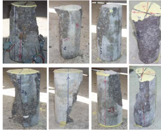
Fig. 9 Fracture patterns of cylinder specimens (Görkem 2012, Zandi and Görkem 2013)
