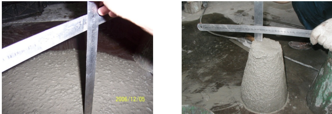
Fig. 3 Comparison of slump between SCC and CVC used in Table 4
