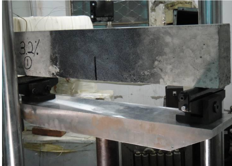
Fig. 3 The FRC specimen with rolling supports
