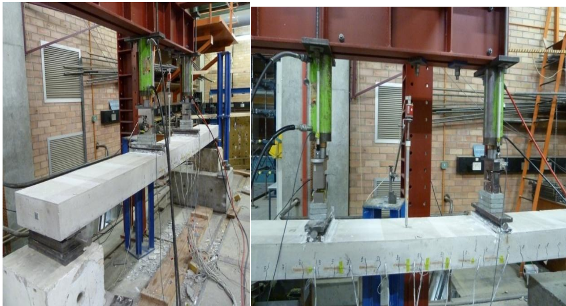
Fig. 3 General view of loading cells, concrete strain gauges, and position sensor test set-up
