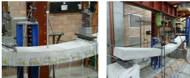
Fig. 6 General view of slab N-SCC-a failure
