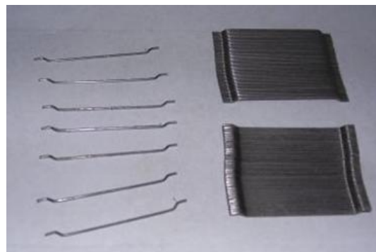
(b) Appearance of the steel fibers
