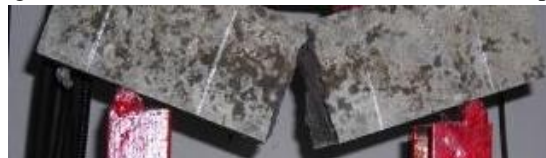
(b) Post-test aspect of the specimens without fibers
