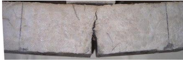
(b) Post-test aspect of the notched SFRC specimen
