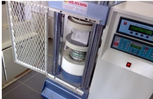
(a) Concrete test press machine (YKM-C205) with 2000 kN capacity
