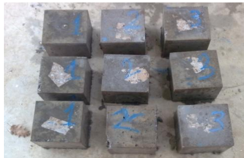
(c) Concrete specimens after cure process
