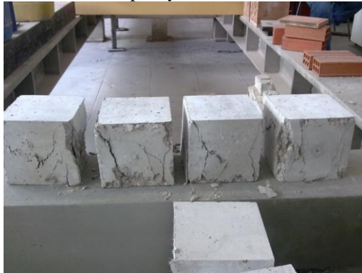
(c) Reference specimens after pressure test
