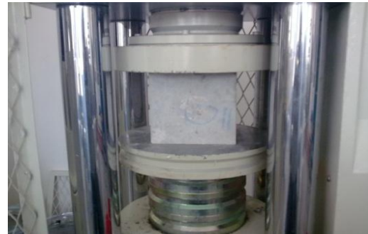
(b) View of the cubic mold during axial pressure test
