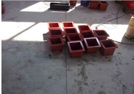
(a) 150 × 150 mm cubic concrete molds
