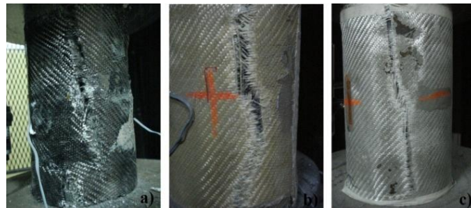
Fig. 7 Failure modes of the FRP-wrapped UHPC columns obtained from the test results (a) GFRP; (b) AFRP ; (c) CFRP
