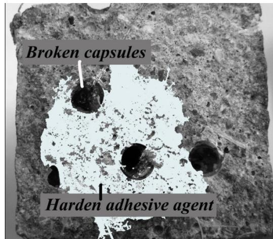
Fig. 8 Broken capsules and harden adhesive agent in the specimens after self-healing
