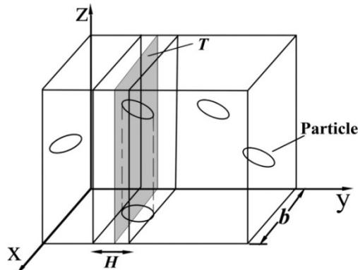
Fig. 5 Intersection between a crack and a capsule
