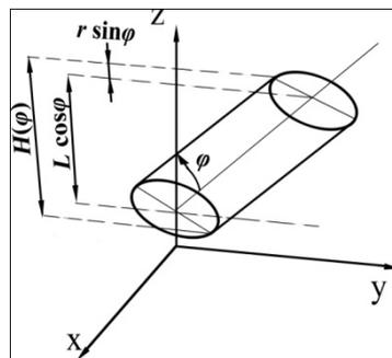
Fig. 6 The caliper diameter ( $H(\varphi)$ ) of a capsule
