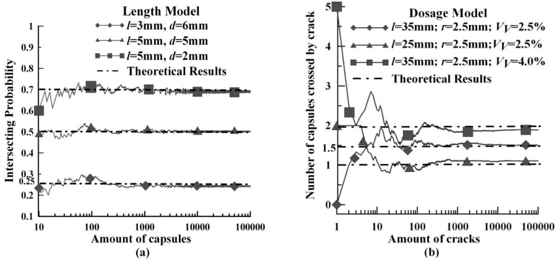
Fig. 7 Simulated results vs. theoretical results: (a) Length model and (b) Dosage model
