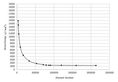
Fig. 4 Diagram of strain energy in terms of element numbers
