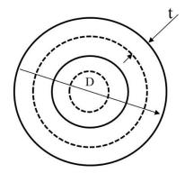
Fig. 1 Cross section of bone scaffold model
