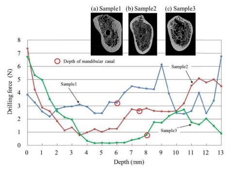
Fig. 2 Results of calculated drilling force with their micro-CT images
