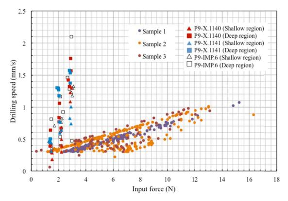
Fig. 7 Results of drilling force and speed on training simulator and polymeric model. The triangular and square markers indicate the results for the polymeric model experiment while the circle marker indicate the three samples evaluated by the clinicians
