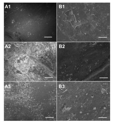
Fig. 5 SEM photos of biodegradable beads right at day 0 (A1, B1), 3 (A2, B2) and 10 (A3, B3) days of elution in the PBS (A: cisplatin at the surface layer, B: 5-FU at the surface layer)
