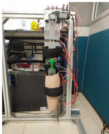
Fig. 3 The upper limb exoskeleton system
