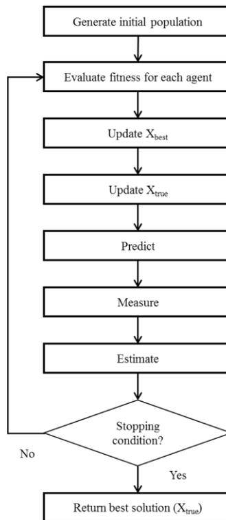
Fig. 2 The SKF algorithm
