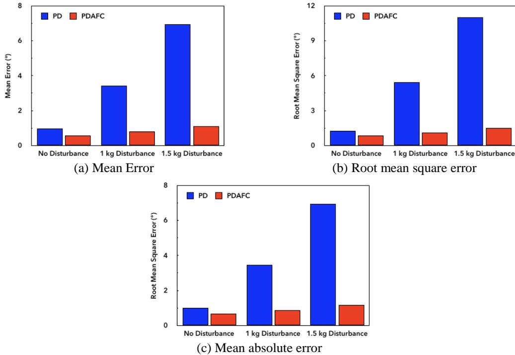
Fig. 5 The tracking performance of the exoskeleton in terms of error metrics
