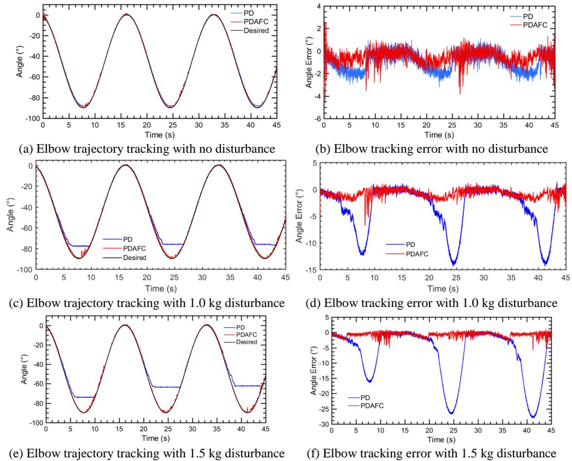
Fig. 4 The trajectory tracking and tracking error of the exoskeleton with and without the influence of mannequin weight as a form of disturbance to the system
