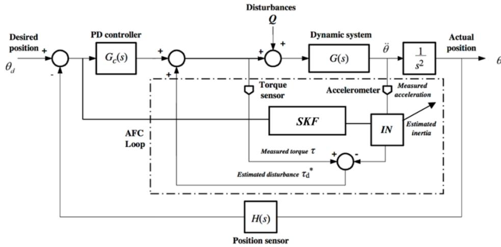
Fig. 1 The PD with SKF based AFC scheme for the control of the upper limb exoskeleton
