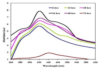
Fig. 2 Absorption spectrum of CdS nanoparticles synthesized by the culture supernatant of *S.nematodiphila* (420 nm)
