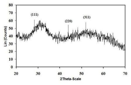
Fig. 4 XRD pattern of synthesized CdS nanoparticles by using S. nematodiphila
