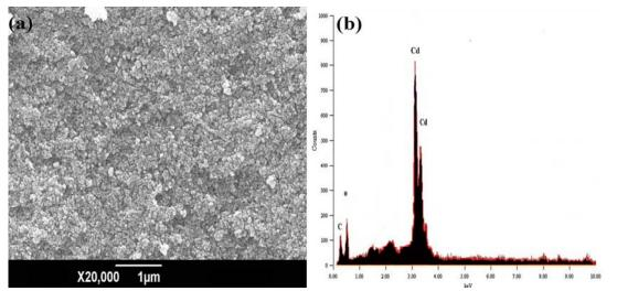
Fig. 5 SEM micrograph of CdS nanoparticles formed after reaction of culture supernatant with 1mM cadmium sulphate for 24hrs (b) Energy Dispersive X-ray of CdS nanoparticle
