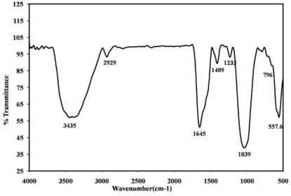
Fig. 3 FTIR spectra recorded from powder of CdS nanoparticles synthesized using S. nematodiphila
