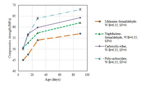
Fig. 13 Variation of compressive strength with time in mixes with W/B=0.35 and SF=0
