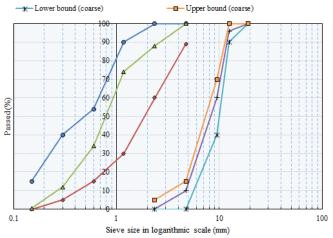
Fig. 2 Grading of coarse and fine aggregates of series B
