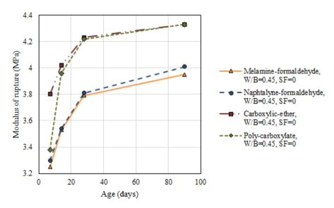
Fig. 18 Variation of rupture modulus with time in mixes with W/B=0.45 and SF/C=0%
