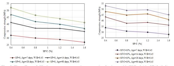
Fig. 8 The effect of SP dosage on compressive strength of mixes with W/B=0.45, SF=0 (left) and SF/C=10% (Right)
