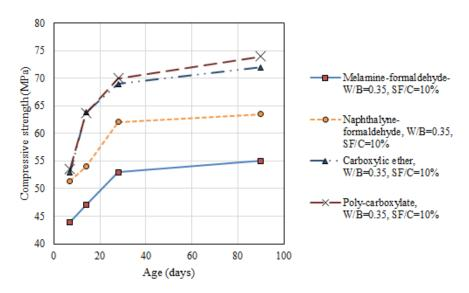
Fig. 14 Variation of compressive strength with time in mixes with W/B=0.35 and SF/C=10%
