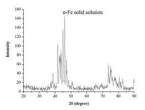
Fig. 2 X-ray diffraction pattern of the gas atomized powder particles
