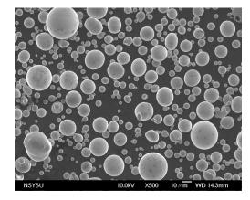
Fig. 3 SEM images of the  $Fe_{50}Cr_{24}Mo_{21}Si_2B_3$  powder particles
