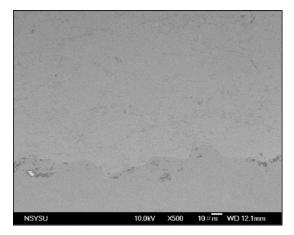
Fig. 5 SEM cross-sectional images of the Fe-based alloy coating
