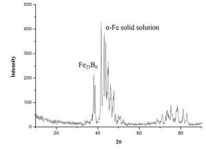
Fig. 1 X-ray diffraction pattern of the  $Fe_{50}Cr_{24}Mo_{21}Si_2B_3$  master ingot
