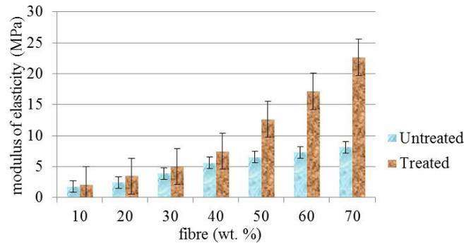
Fig. 2 Modulus of elasticity of oil palm EFB reinforced polyester reinforced composites at different fibre loading
