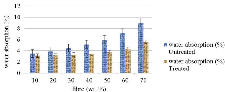
Fig. 4 Water absorption of oil palm EFB reinforced polyester reinforced composites at different fibre loading
