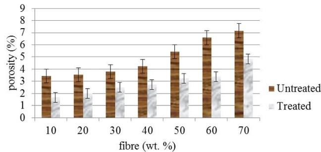
Fig. 3 Porosity of oil palm EFB reinforced polyester reinforced composites at different fibre loading
