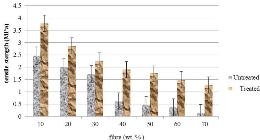
Fig. 1 Tensile strength of oil palm EFB reinforced polyester reinforced composites at different fibre loading
