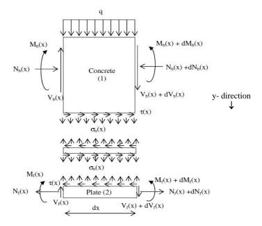
Fig. 2 Forces in infinitesimal element of a soffit-plated beam
