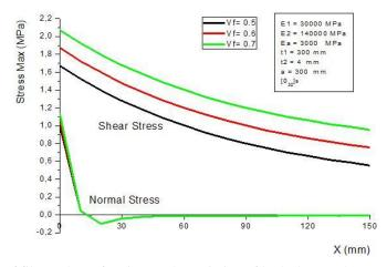
Fig. 11 The effect of fiber volume fraction on the variation of both shear and normal adhesive stresses in RC beam bonded with composite plate
