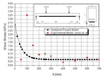
Fig. 4 Comparison of interfacial shear of the steel plated RC beam with the experimental results
