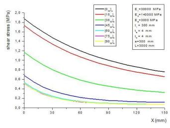
Fig. 10 Effect of the fiber orientation on the interfacial shear stresses for RC beam with a bonded CFRP soffit plate
