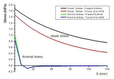
Fig. 5 Comparison of interfacial shear and normal stresses for an RC beam with a bonded CFRP soffit plate subjected to a uniformly distributed load (without creep and shrinkage effect)
