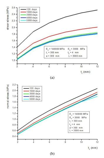
Fig. 8 (a) Effect of maximum edge shear stress with different thickness of CFRP; (b) Effect of maximum edge normal stress with different thickness of CFRP
