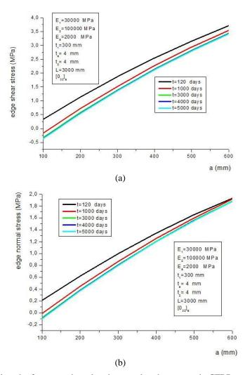
Fig. 9 (a) Influence of length of unstrengthened region on edge shear stress in CFRP strengthened RC beam;(b) Influence of length of unstrengthened region on edge normal stress in CFRP strengthened RC beam
