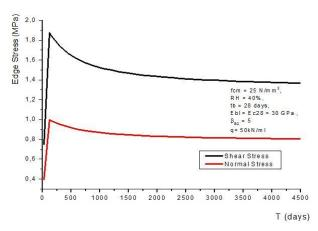
Fig. 6 Time development of interfacial edge stresses for an RC beam with a bonded CFRP soffit plate
