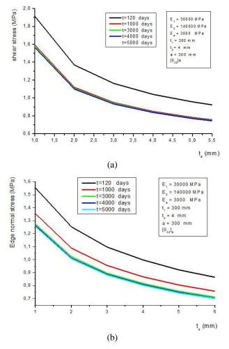
Fig. 7 (a) Effect of adhesive layer thickness on edge shear stresses in CFRP strengthened RC beam;(b) Effect of adhesive layer thickness on edge normal stresses in CFRP strengthened RC beam
