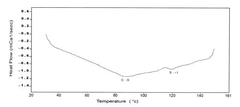
Fig. 6 DSC Thermmogram of PPy-Red-II; the traces were obtained on heating from the crystalline to semectic phase  $(C \rightarrow S)$  and semectic to isotropic phase  $(S \rightarrow I)$  at the heating rate 10 min<sup>-1</sup>
