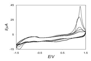
Fig. 2 Cyclic voltammograms of PPy-Red-II-co-Py formation [(Py-Red-II (1 mmol) and Pyrrole (0.5 mmol)], LiClO<sub>4</sub> (0.1 M) in 20 mL acetonitrile on GC disk electrode vs. Ag/AgCl reference electrode,  $v = 50 \text{ mVs}^{-1}$  (10 cycles)
