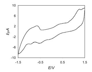
Fig. 3 Cyclic voltammogram of PPy-Red-II-co-Py on a GC disk electrode vs. Ag/AgCl reference electrode in  $LiClO_4$  (0.1 M) in 20 mL acetonitrile,  $v = 50 \text{ mVs}^{-1}$
