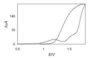
Fig. 1 Cyclic voltammogram of Py-Red-II (1 mmol) on a GC disk electrode vs. Ag/AgCl reference electrode and LiClO<sub>4</sub> (0.1 M1) in 20 mL acetonitrile,  $v = 50 \text{ mVs}^{-1}$
