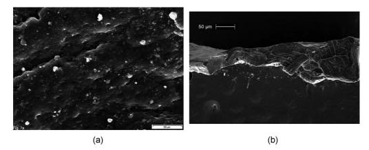
Fig. 8 SEM Micrographs of PPy-Red-II: (a) surface and (b) cross section images
