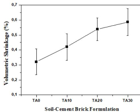
Fig. 3 Volumetric shrinkage of the soil-cement bricks
