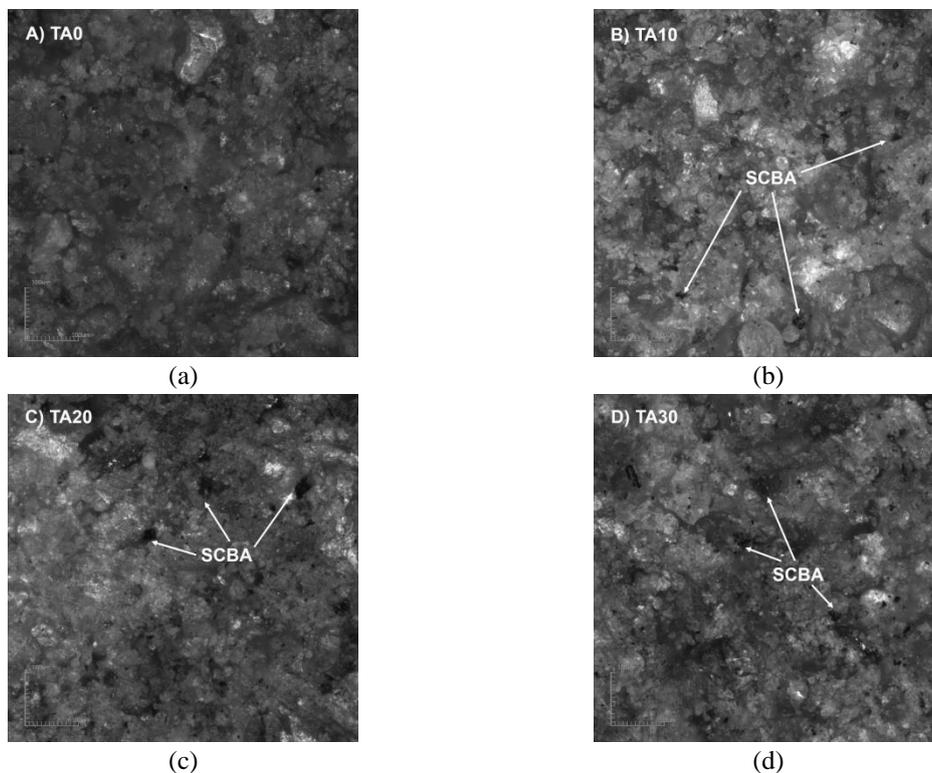
Fig. 2 Confocal micrographs of the cured soil-cement bricks
