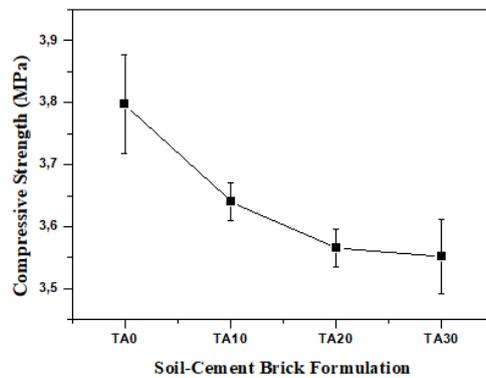
Fig. 6 Compressive strength of the soil-cement bricks
