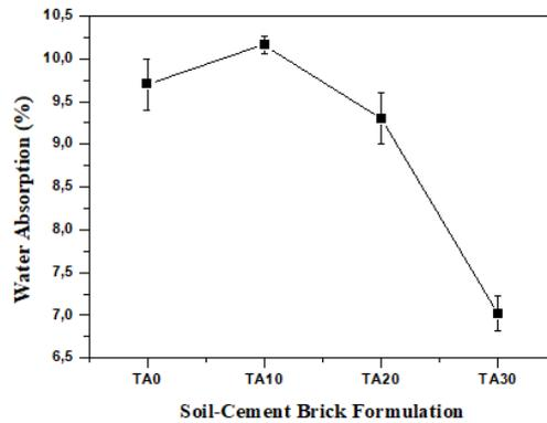
Fig. 5 Water absorption of the soil-cement bricks
