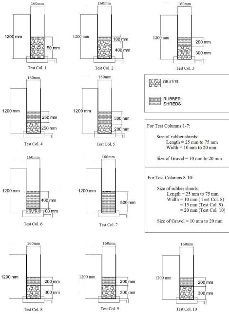
Fig. 2 Schematic representation of experimental test cols. 1-10
