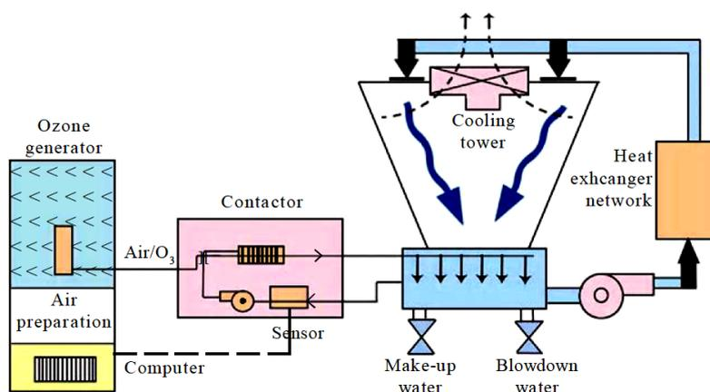
Fig. 1 A schematic of integrating ozone treatment into the cooling tower
