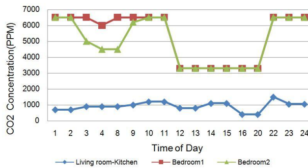
Fig. 5 CO 2 concentration during day in the living room and bedrooms in winter season
