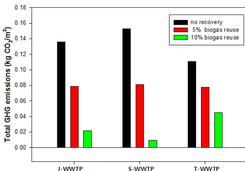
Fig. 5 Total GHG emissions with and without biogas recovery and reuse
