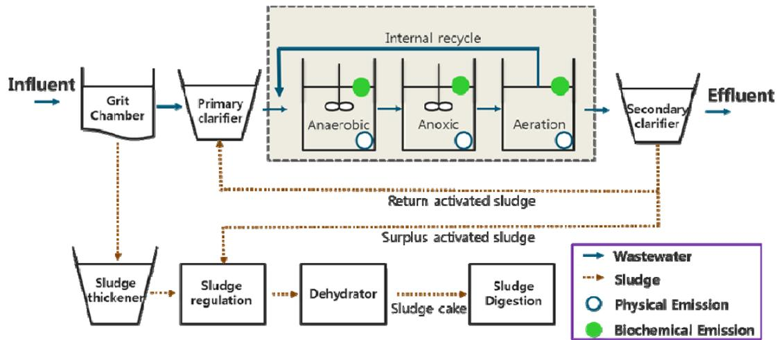
Fig. 1 Flow diagram of hybrid WWTP and system boundary for the estimation of GHG emissions
