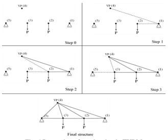
Fig. 4 Prevention of overlapping in TUBM
