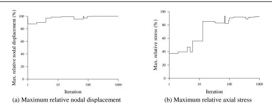
Fig. 12 Relative deflection and stress histories for size, shape and topology optimization of the 11-members, 6-nodes truss structure with TUBM and iPSO
