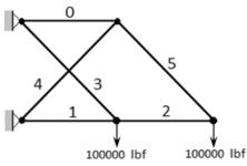
Fig. 10 Optimized structural configuration of the 11-members, 6-nodes truss system found with TUBM and iPSO
