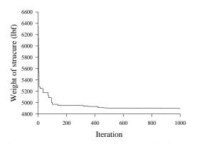
Fig. 11 Weight convergence history for size, shape and topology optimization of the 11-members, 6-nodes truss structure with TUBM and iPSO
