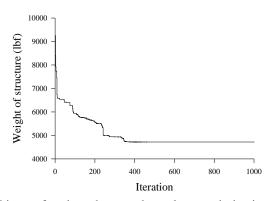
Fig. 7 Weight convergence history for size, shape and topology optimization of the 15-members, 6-nodes truss structure with GSM and iPSO
