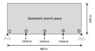
Fig. 14 Geometric search space for two-tire planar truss structure with extra 7 variable points
