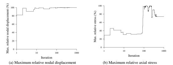
Fig. 8 Relative deflection and stress histories for size, shape and topology optimization of the 15-members, 6-nodes truss structure with GSM and iPSO
