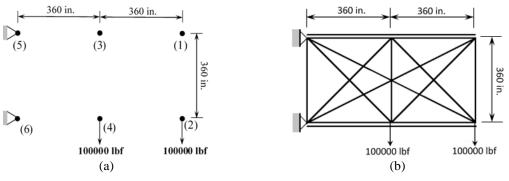
Fig. 5(a) Initial system, (b) Ground structure generated using GSM
