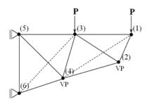
Fig. 3 A sample structure generated by TUBM with two variable points (VPs) and two free elements
