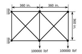
Fig. 9 Ground structure manually generated (Deb and Gulati 2001, Ringertz 1985)
