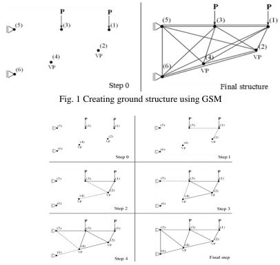
Fig. 2 Creating ground structure using TUBM
