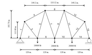
Fig. 15 Optimized structural configuration of the two-tire planar truss system found with TUBM and iPSO
