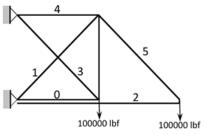
Fig. 6 Optimized structural configuration of the 15-members, 6-nodes truss system found with GSM and iPSO
