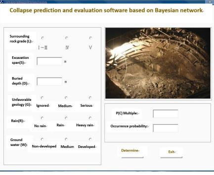
Fig. 5 Collapse prediction software based on Bayesian network
