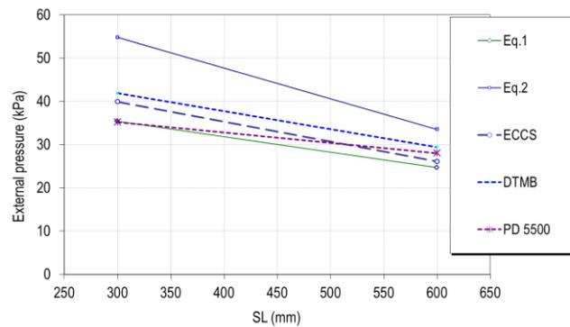
Fig. 3 Estimations of critical loads obtained from design codes and recommendations
