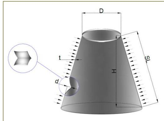
(b) geometry of conical shell under external pressure
