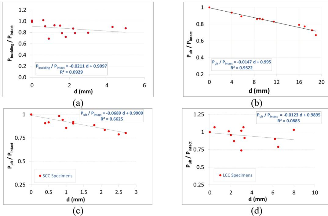
Fig. 7 Capacity ratio of the dented to the intact specimens (Ghanbari Ghazijahani *et al.* December 2015): (a) slender shells under external pressure (Ghanbari Ghazijahani *et al.* 2014), (b) tubes under compression (Ghanbari Ghazijahani *et al.* 2015), (c,d) slender shells under compression (Ghanbari Ghazijahani *et al.* 2014)
