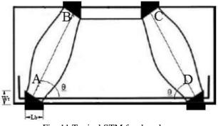
Fig. 11 Typical STM for deep beam
