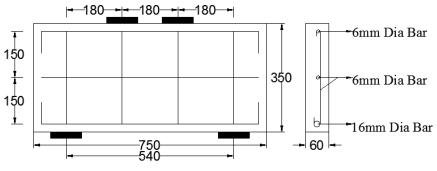
Fig. 4 Typical reinforcement details of deep beam
