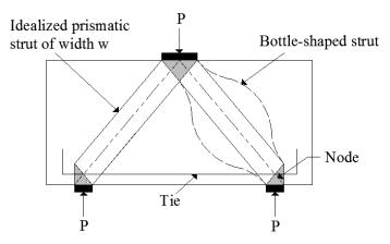
Fig. 1 STM for deep beam with central point load
