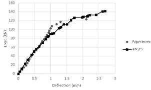
Fig. 6 Load Deflection Plot for Beam E1
