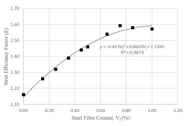
Fig. 12 Plot showing variation of efficiency factor with steel fibre ratio
