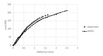
Fig. 9 Load deflection plot for beam E4
