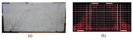
Fig. 10 Crack pattern for beam E1 (a) From Experiment (b) From ANSYS
