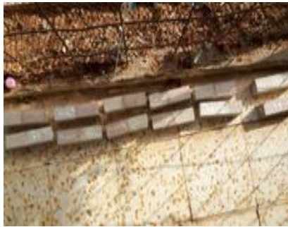
Fig. 2 Prism samples curing in hot climate
