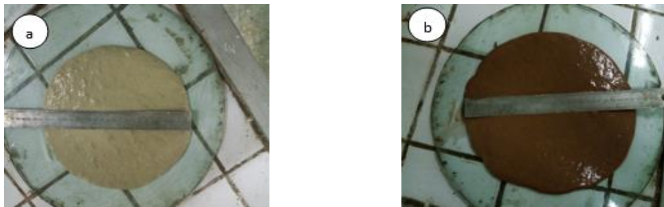
Fig. 4 Photographs of mortar slump flow: (a) SCM-00NP and (b) SCM-40NP
