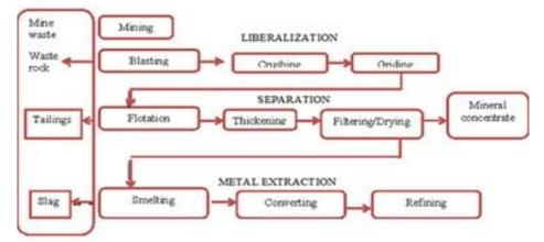
Fig. 1 Mineral extraction from mining to metal (Spitz and Trudinger 2009)
