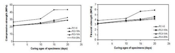
Fig. 16 Compressive strength with waste plastic Fig. 17 Flexural strength with waste plastic (Zainab (Zainab *et al.* 2008) *et al.* 2008)
