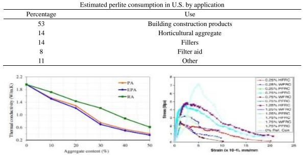
Fig. 14 Effect of EPA, PA and RA content on the Fig. 15 Flexural strength vs. strain for fiber thermal conductivity (Oktay *et al.* 2015) reinforced concretes (Gul *et al.* 2007)
