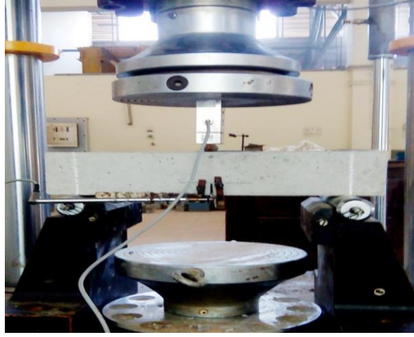
Fig. 3 Actual test setup for single point loading test
