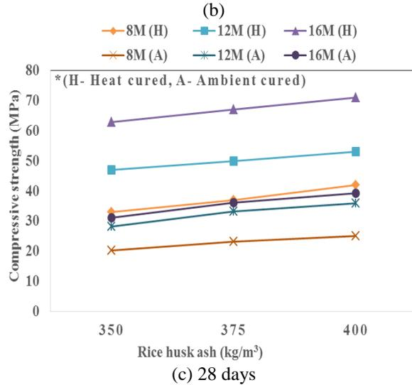
Fig. 6 Compressive strength of RHA based GPC
