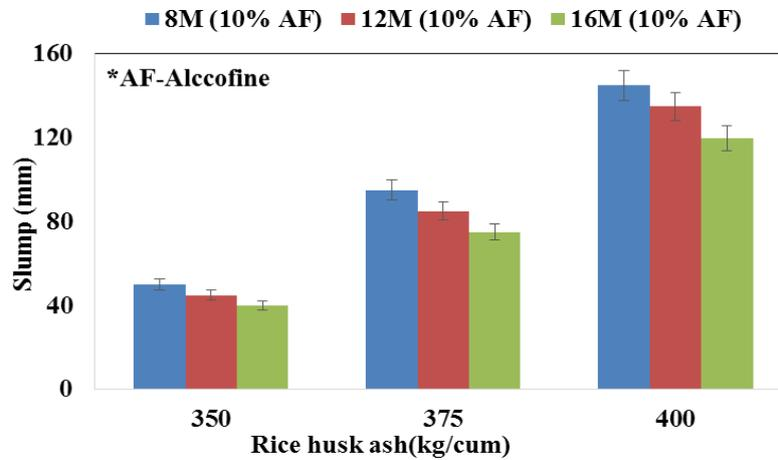
Fig. 4 Slump of GPC mixes with varying RHA content
