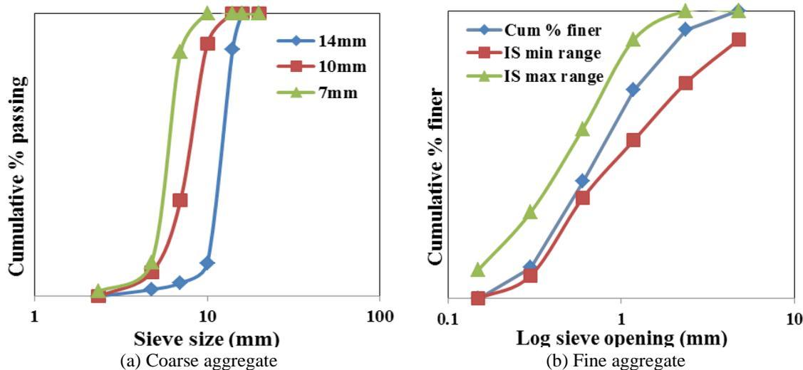
Fig. 3 Grading curve of (a) Coarse aggregate (b) Fine aggregate
