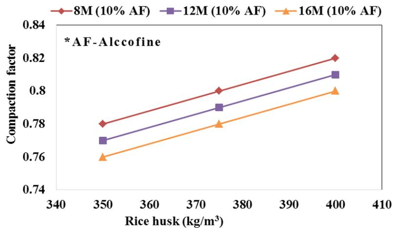
Fig. 5 Compaction factor of GPC mixes with different RHA content
