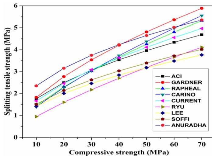
Fig. 9 Relationship between compressive and splitting tensile strength at 28 days
