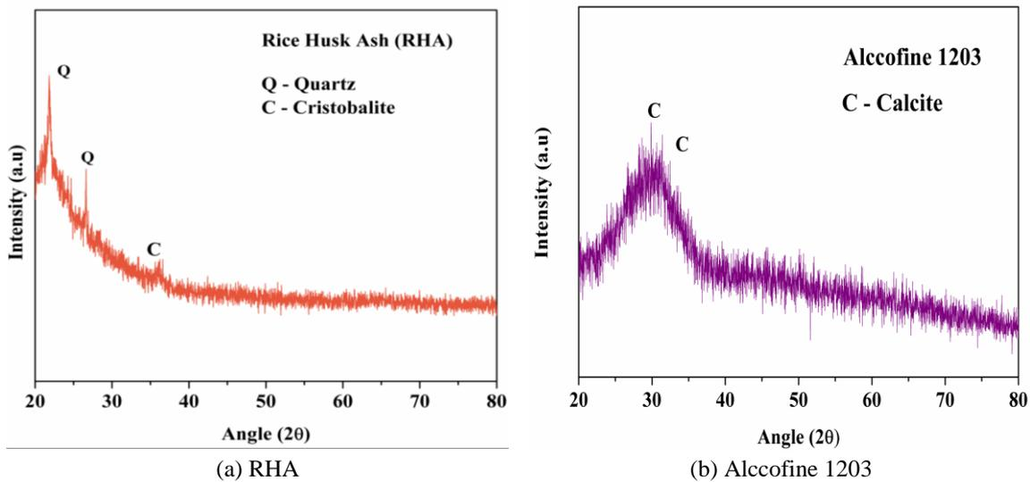
Fig. 2 XRD spectrum of RHA and Alccofine 1203
