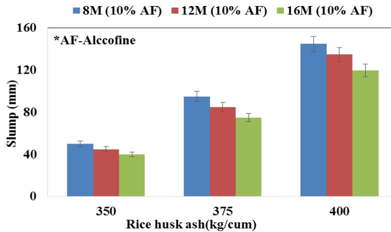
Fig. 4 Slump of GPC mixes with varying RHA content
