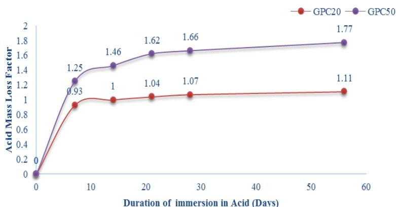
Fig. 8 Acid mass loss factor vs. Duration of immersion in acid
