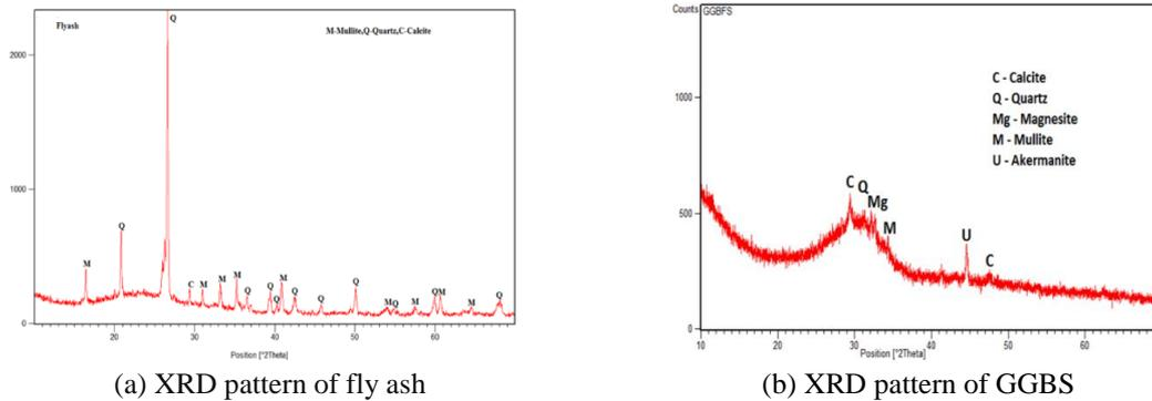
Fig. 3 XRD pattern of fly ash and GGBS
