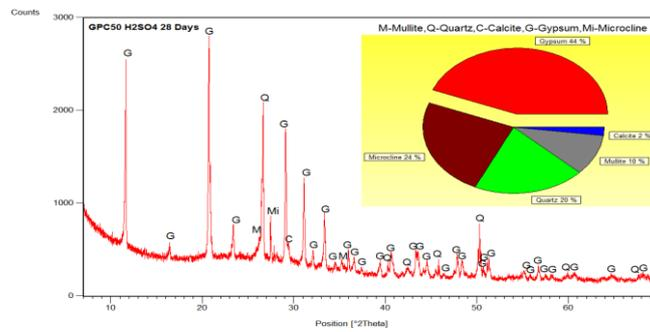
Fig. 14 XRD analysis for specimens subjected to H<sub>2</sub>SO<sub>4</sub> for 28 days (GPC50)
