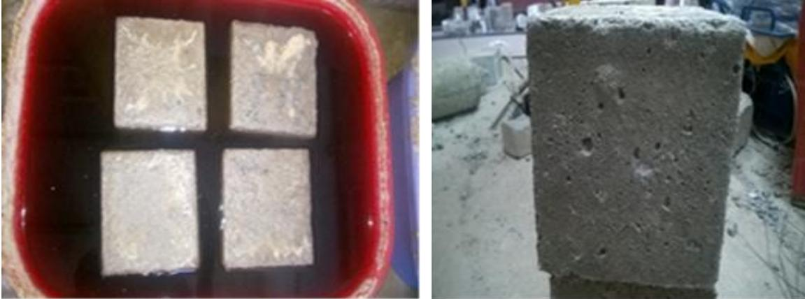
Fig. 7 Visual of specimens subjected to  $H_2SO_4$  of GPC20 and GPC50 after 56 days
