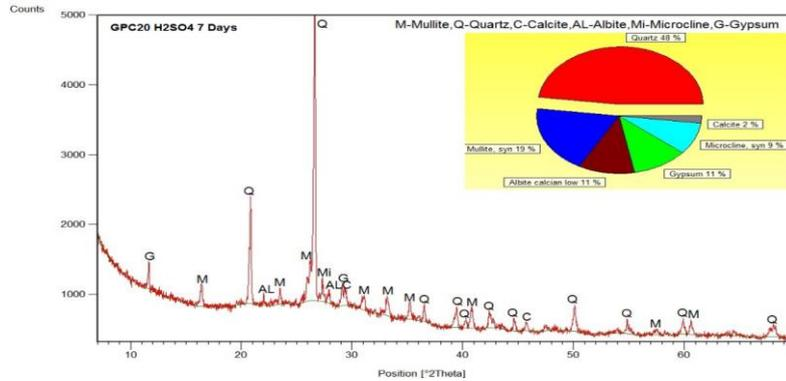
Fig. 10 XRD analysis for specimens subjected to H<sub>2</sub>SO<sub>4</sub> for 7 days (GPC20)
