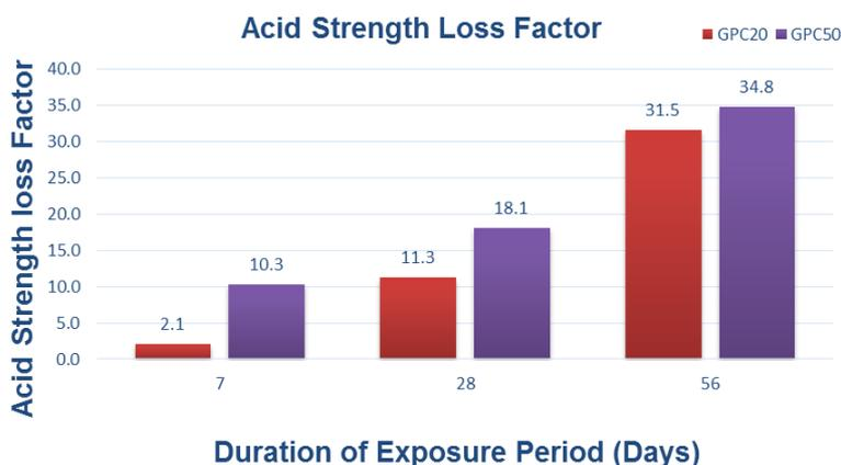
Fig. 9 Acid strength loss factor vs. Duration of immersion in acid
