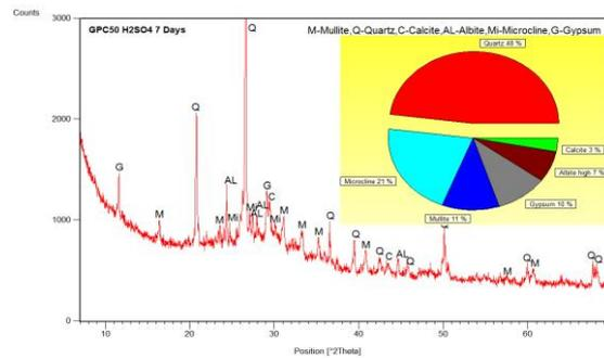
Fig. 13 XRD analysis for specimens subjected to H<sub>2</sub>SO<sub>4</sub> for 7 days (GPC50)
