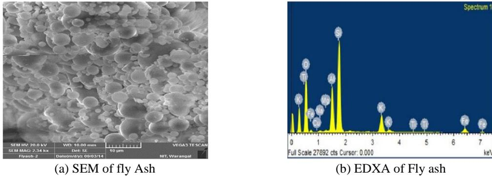
Fig. 1 SEM and EDXA of fly Ash
