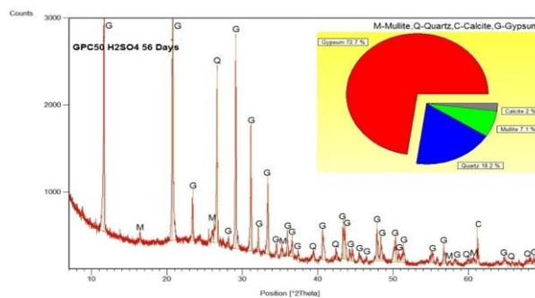
Fig. 15 XRD analysis for specimens subjected to H<sub>2</sub>SO<sub>4</sub> for 56 days (GPC50)
