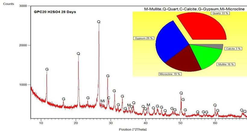
Fig. 11 XRD analysis for specimens subjected to H<sub>2</sub>SO<sub>4</sub> for 28 days (GPC20)
