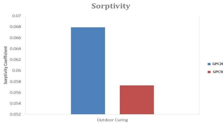
Fig. 6 Sorptivity of ambient-cured geopolymer concrete at 28-days for GPC20 and GPC50
