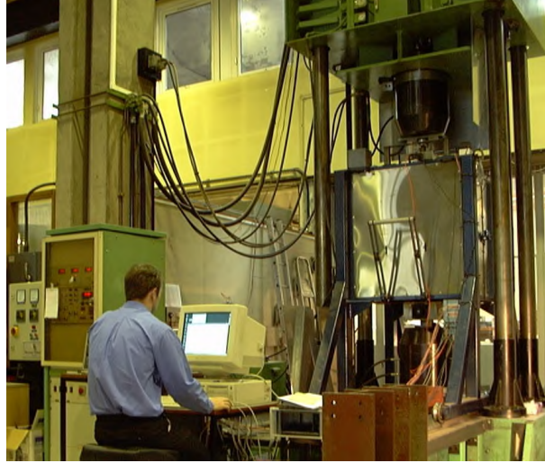
Fig. 1 A programme-controlled furnace with the 2000 kN LOS testing machine
