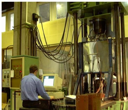
Fig. 2 A programme-controlled furnace in the 2000 kN LOS testing machine
