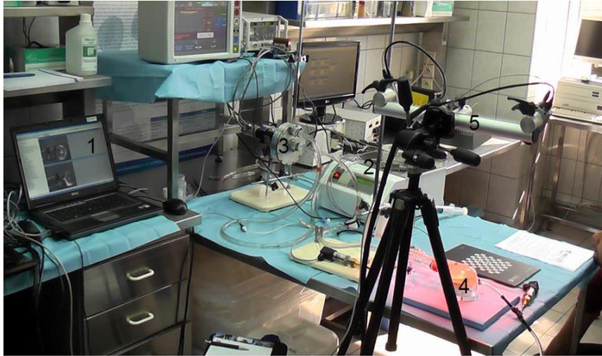
Fig. 2 An overview of the DIC experimental setup: 1 – PC and electronic system, 2 – tank and temperature stabilising system, 3 – centrifugal pump, 4 – pneumatic pump, and 5 – cameras
