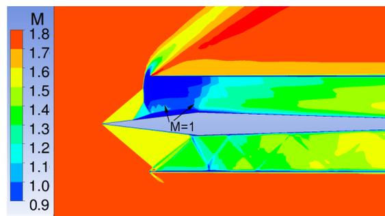
Fig. 13 Mach number contours in 2D flow over the longer centerbody. The same asymmetric flow regime at  $M_\infty=1.8$ ,  $\alpha=0$  as in Fig. 5
