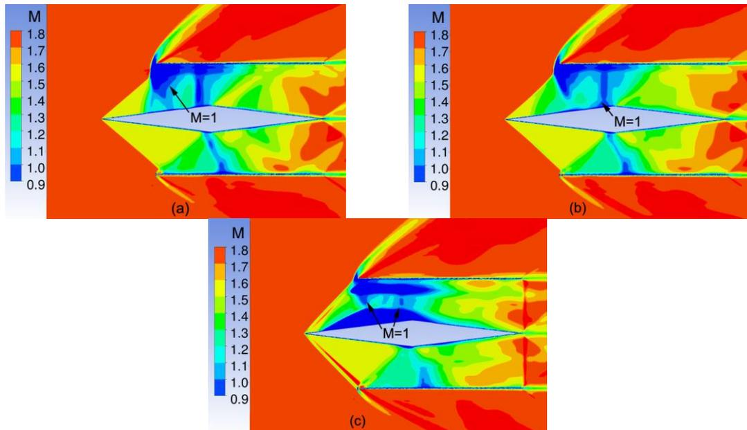
Fig. 12 Mach number contours in span sections of the 3D flow shown in Fig. 11: (a)  $z=0$ , (b)  $z=0.075$ , (c)  $z=0.14$
