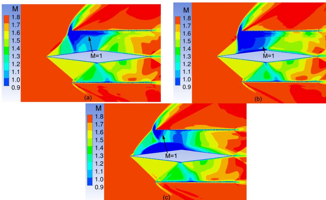
Fig. 9 Mach number contours in span sections of the 3D flow shown in Fig. 8: (a)  $z=0$ , (b)  $z=0.15$ , (c)  $z=0.25$
