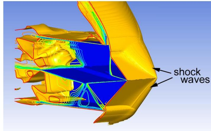
Fig. 8 Mach number contours in the plane  $z=0$  and isosurfaces  $M(x, y, z)=1.7$  over the 3D centerbody and channel of half-span  $0 < z < 0.3$ . The same asymmetric flow regime at  $M_\infty=1.8$ ,  $\alpha=0$  as in Fig. 5
