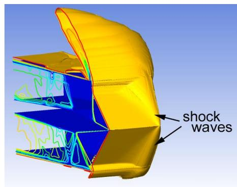
Fig. 14 Mach number contours in the plane  $z=0$  and isosurfaces  $M(x, y, z)=1.7$  in/over a longer channel of half-span  $0 < z < 0.3$ . The same asymmetric flow regime at  $M_\infty=1.8$ ,  $\alpha=0$  as in Fig. 5
