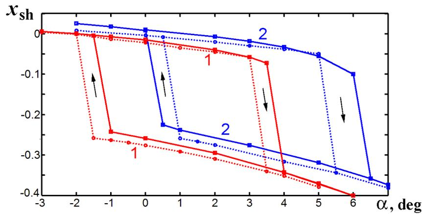
Fig. 6 Coordinate  $x_{sh}$  of a shock wave generated by the bow of the lower wall versus the angle of attack  $\alpha$ . Curves 1:  $M_\infty=1.85$ , curves 2:  $M_\infty=1.95$ . Solid curves – computations with ANSYS-15 CFX, dashed curves – computations with ANSYS-15 Fluent density-based solver
