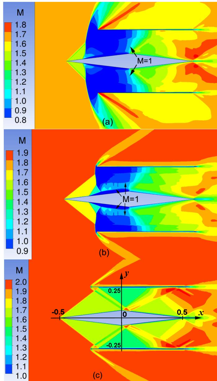
Fig. 4 Mach number contours in symmetric 2D flow at the vanishing angle of attack  $\alpha=0$ : (a)  $M_\infty=1.65$ , (b)  $M_\infty=1.88$ ; the solution is obtained by increasing  $M_\infty$  from 1.65 to 1.88, (c)  $M_\infty=1.92$
