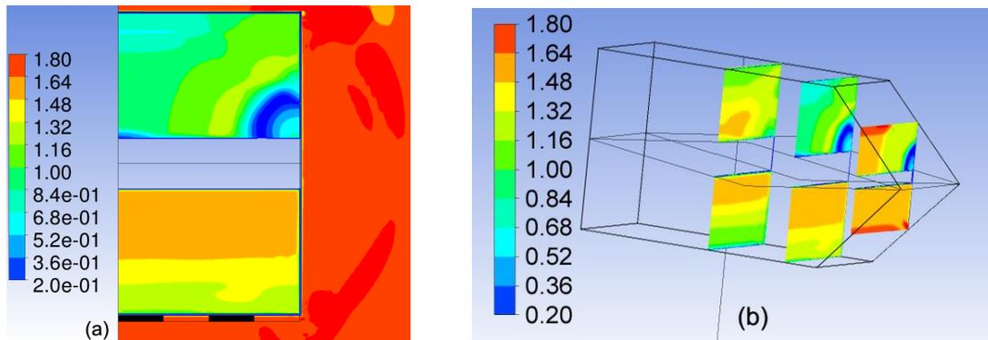
Fig. 10 Mach number contours in cross sections of the 3D flow shown in Fig. 8: (a)  $x = -0.15$ , (b)  $x = 0.1, -0.15, -0.35$
