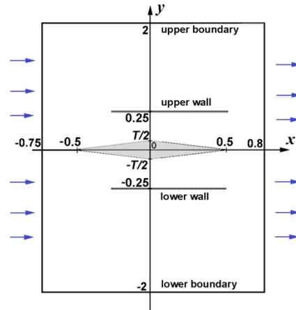
Fig. 2 Schematic of the computational domain
