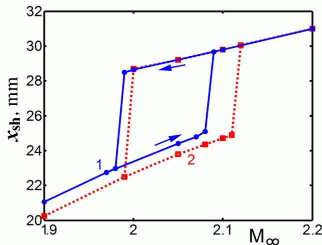
Fig. 7 Coordinate  $x_{sh}$  of the oblique shock at the height of 9.5 mm in the intake shown in Fig. 3: 1 – original intake (Das and Prasad 2010) with the smoothed lower wall at the throat; 2 – modified intake with a corner of the lower wall profile at the throat
