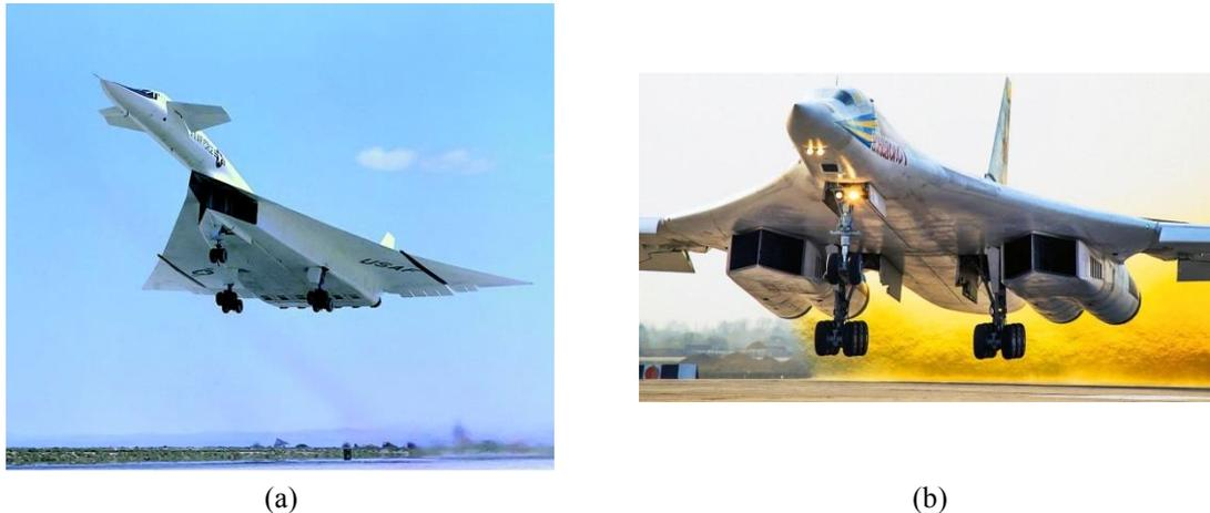
Fig. 1 Twin intakes used in jets: (a) North American XB – 70 Valkyrie (Wikipedia 2017), (b) Russian TU-160 Blackjack (Военное обозрение 2018)
