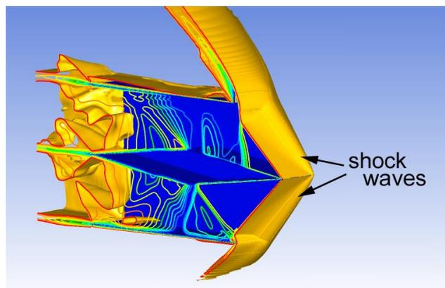
Fig. 11 Mach number contours in the plane  $z=0$  and isosurfaces  $M(x, y, z)=1.7$  over the 3D centerbody and channel of the reduced half-span  $0 < z < 0.15$ . The same asymmetric flow regime at  $M_\infty=1.8$ ,  $\alpha=0$  as in Fig. 5
