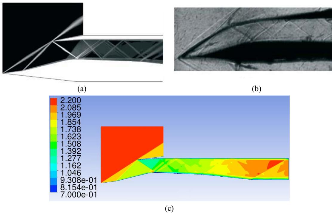
Fig. 3 An intake used for the solver validation. Mach number contours at  $M_\infty=2.2$  and cowl deflection angle of 4 deg: (a) and (b) numerical simulations and experimental data, respectively, reproduced from (Das and Prasad 2010) with permission; (c) our computations with ANSYS-15 CFX. The length of the channel displayed in (c) is 119 mm
