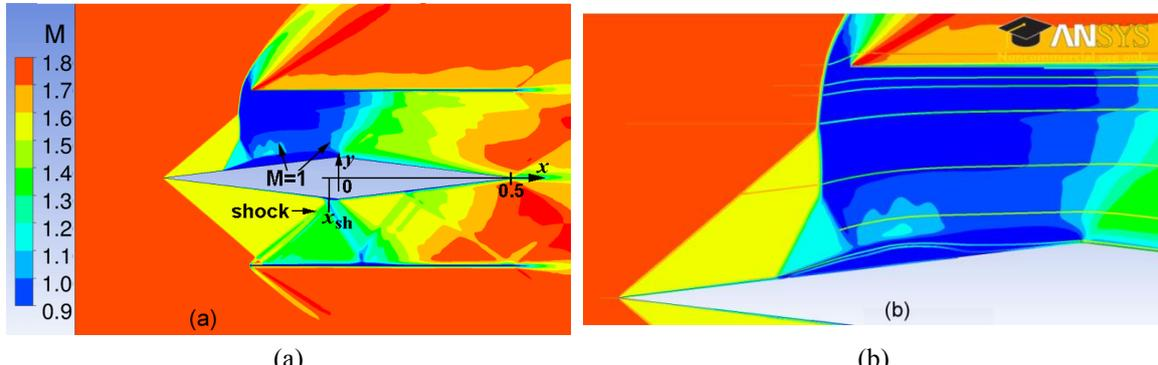
Fig. 5 Asymmetric 2D flow with an expelled shock in the upper part of the channel and a train of shocks in the lower part,  $M_\infty=1.8$ ,  $\alpha=0$ : (a) Mach number contours; (b) streamlines in the region of boundary-layer separation
