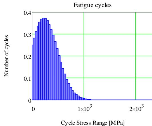
Fig. 5 Example Cycle stress range histogram using Lalanne approach
