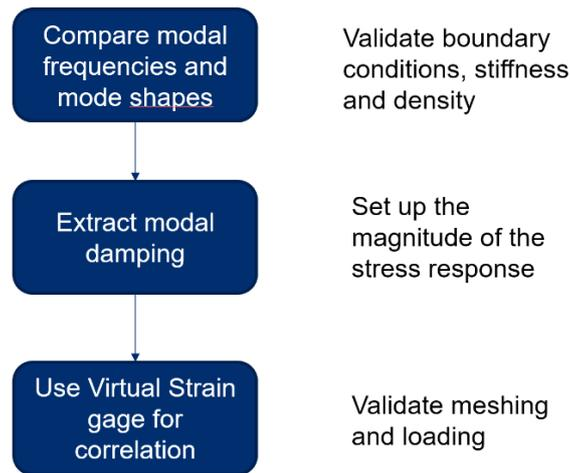
Fig. 9 Summary diagram for the validation of a dynamic FE model for stress and fatigue analysis
