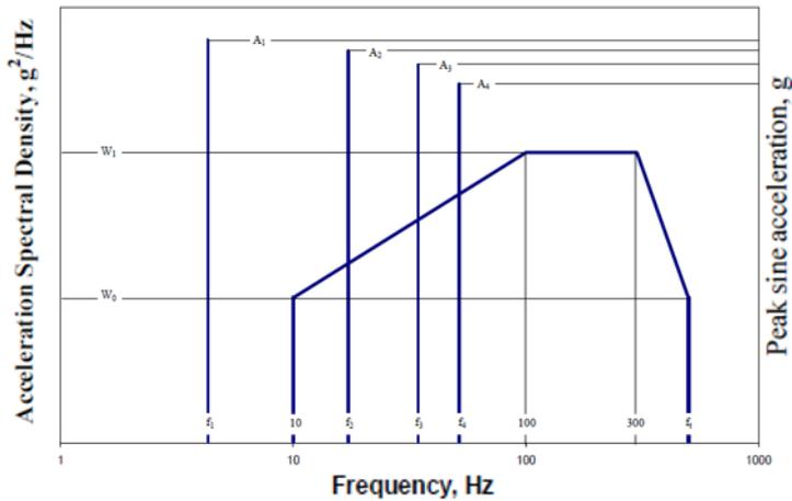
Fig. 2 Example test specification - Helicopter vibrations exposure - MIL STD 810G Figure 514.6C-8
