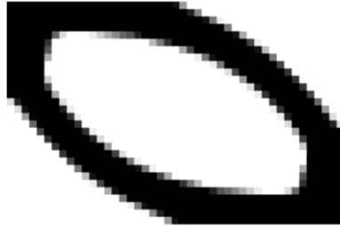
Fig. 5 A new composite design for the rectangular plate with increased first frequency
