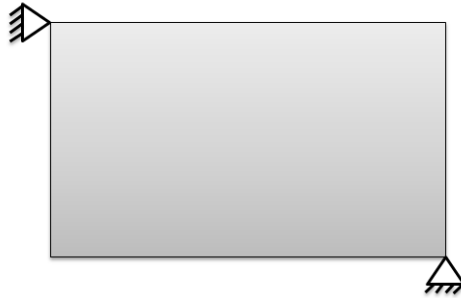
Fig. 3 Rectangular plate under plane stress conditions
