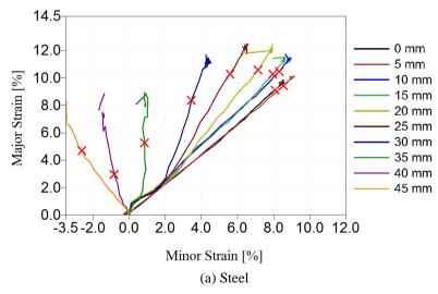
Fig. 8 Graphs of major strains against minor strains at different points along  $0^{\circ}$  meridians of (a) steel and (b) FML samples stamp formed with 14 kN BHF, until maximum load. Strains at forming depth of 30 mm are marked with crosses
