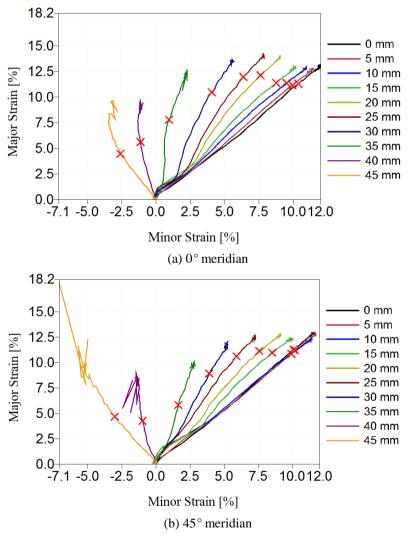
Fig. 6 Major strains against minor strains at different points along (a)  $0^{\circ}$  meridian and (b)  $45^{\circ}$  meridian of an FML stamp formed with 14kN BHF, until maximum load. Strains at wrinkling depth are marked with crosses
