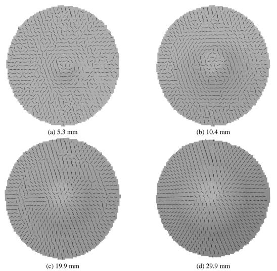
Fig. 10 Direction of major strains shown as lines distributed over the FML specimen stamp formed with 14 kN BHF, at depths of (a) 5.3 mm, (b) 10.4 mm, (c) 19.9 mm and (d) 29.9 mm
