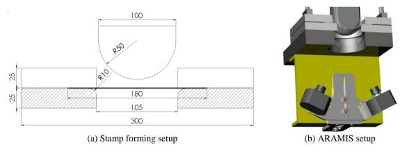
Fig. 3 Stamp forming experimental setup: (a) Cross section the punch, blank holder, blank and the die (Davey 2012), (b) positioning of ARAMIS cameras under the stamping press (Venkatesan 2012)
