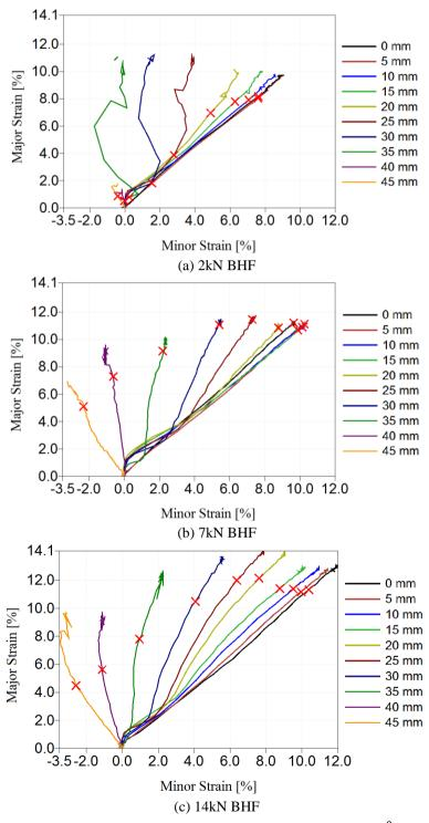
Fig. 9 Major strains plotted against minor strains at different points along  $0^0$  meridians of FML samples stamp formed with a) 2kN, b) 7kN and c) 14kN BHFs, until maximum load. Strains at wrinkling depth are marked with crosses
