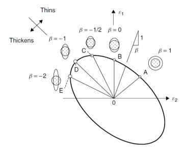
Fig. 7 The strain diagram showing the different deformation modes corresponding to different strain ratios. From right, equibiaxial stretching ( $\beta$ =1), in plane strain ( $\beta$ =0), uniaxial extension ( $\beta$ =-1/2), drawing or pure shear ( $\beta$ =-1) and uniaxial compression ( $\beta$ =-2). (Marciniak 2002)
