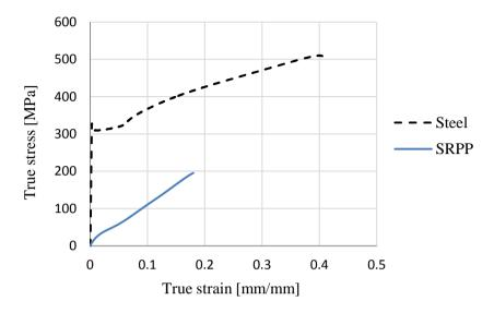
Fig. 2 Stress-strain curves of steel and SRPP along 0°/90° fibre directions
