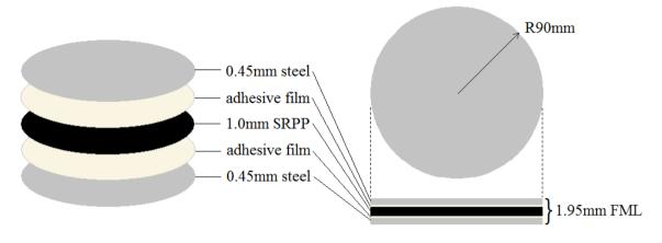
Fig. 1 Steel/SRPP FML blank layup and dimensions
