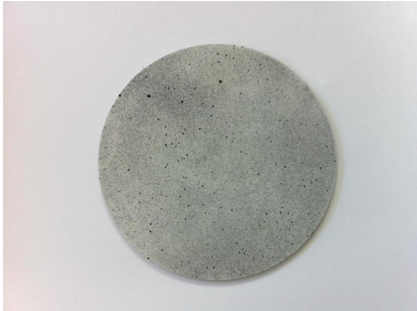
Fig. 2 Stochastic pattern on circular composite material sample (Venkatesan 2012)
