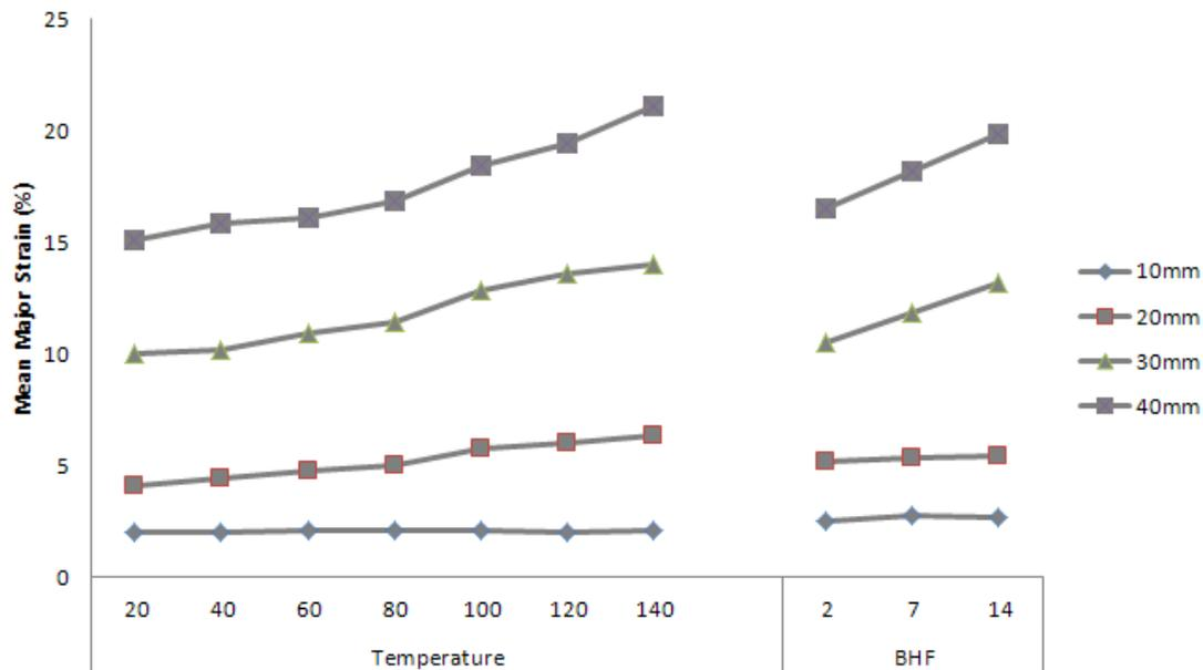
Fig. 8 Main effect of process parameters on mean major strain at point 3 (Venkatesan 2012)
