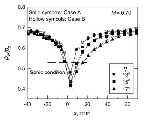
Fig. 3 Wall pressure distributions, transonic interactions
