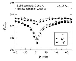
Fig. 2 Wall pressure distributions, subsonic expansion flows
