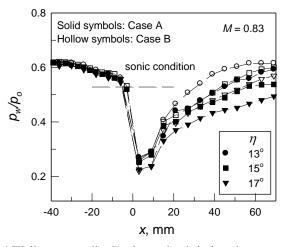
Fig. 4 Wall pressure distributions, shock-induced separated flows
