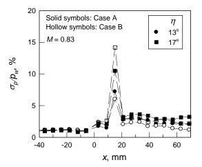
Fig. 7 Surface pressure fluctuations, shock-induced separated flows
