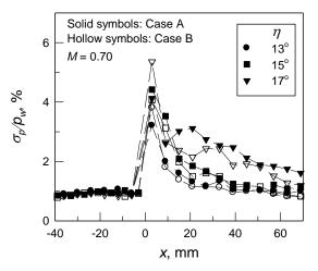
Fig. 6 Surface pressure fluctuations, transonic interactions
