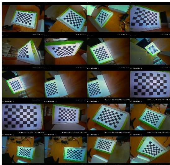
Fig. 1 The images used for calibration
