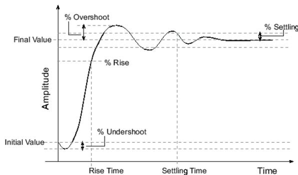
Fig. 22 Step response characteristics (Mathworks 2016)
