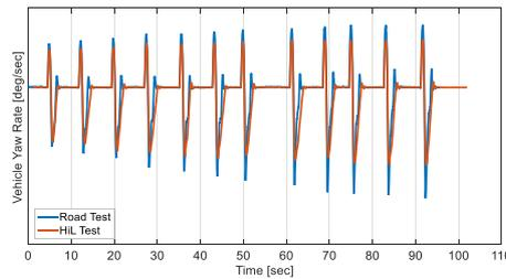
Fig. 13 Change of vehicle yaw rate over time for FMVSS No. 126
