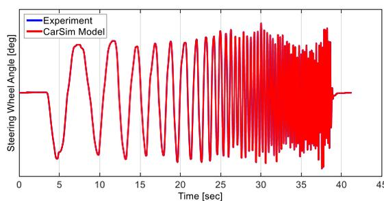
Fig. 3 Steering input in frequency sweep test
