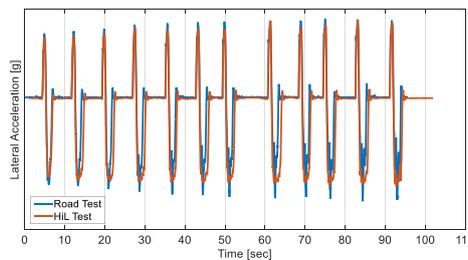
Fig. 14 Change of vehicle lateral acceleration over time for FMVSS No. 126
