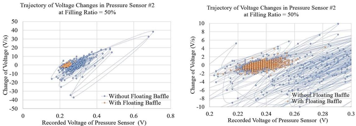
Fig. 13 Trajectory of voltage changes by pressure sensor at location S2 under sloshing by excitation with amplitude = 3.0 cm, period = 1.1 sec, and filling ratio 50%, (left) full view, and (right) zoom in view
