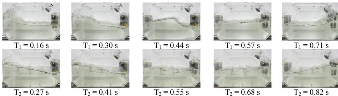
Fig. 6 First half-cycle of sloshing under excitation with amplitude = 3.0 cm, period = 1.1 sec, and filling ratio 50%, (upper) without floating baffle, and (bottom) with floating baffle
