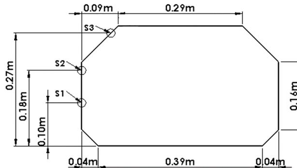
Fig. 3 Principal dimensions of model tank and location of sensors (S1-S3) from front view
