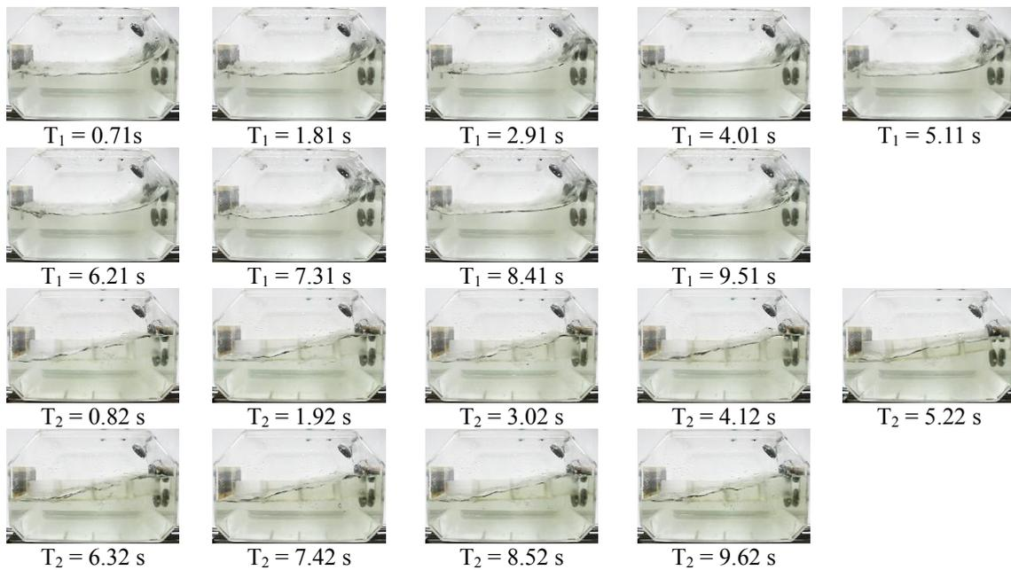
Fig. 8 First nine peaks of sloshing under excitation with amplitude = 3.0 cm, period = 1.1 sec, and filling ratio 50%, (upper) without floating baffle, and (bottom) with floating baffle
