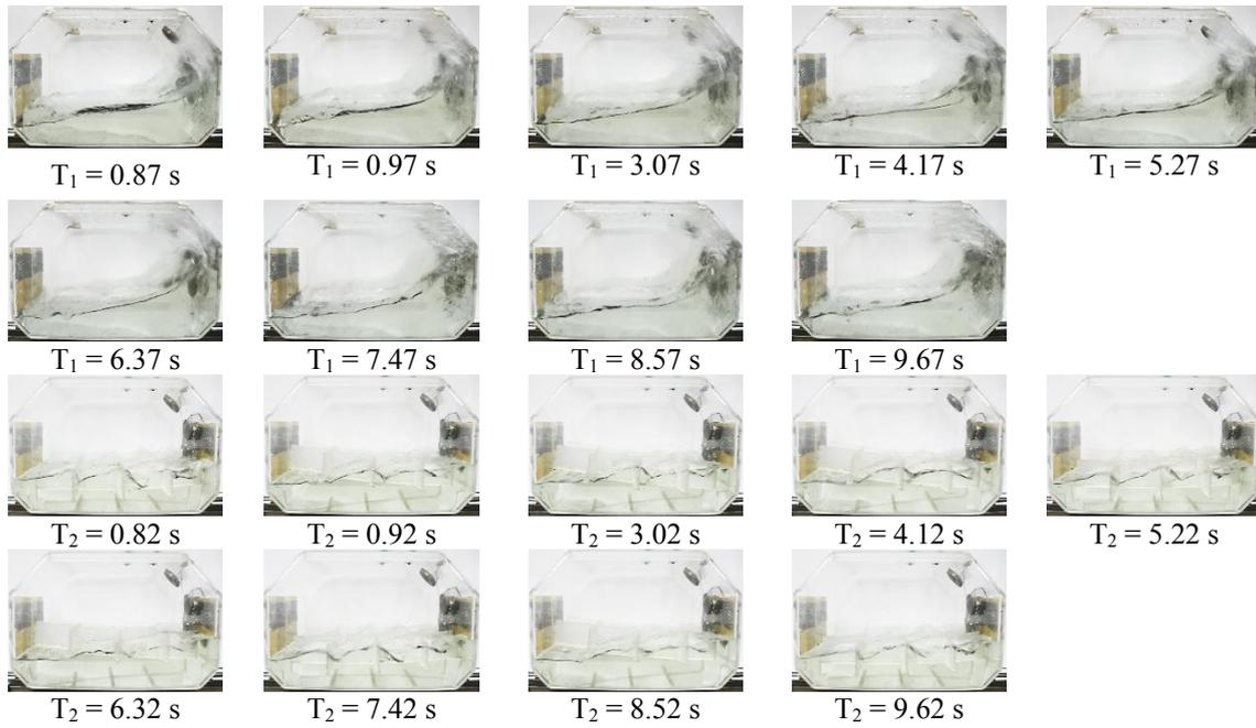
Fig. 7 First nine peaks of sloshing under excitation with amplitude = 3.0 cm, period = 1.1 sec, and filling ratio 30%, (upper) without floating baffle, and (bottom) with floating baffle
