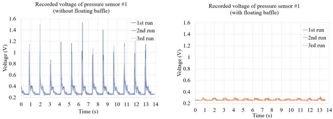
Fig. 10 Voltage recorded by pressure sensor at location s1 under sloshing by excitation with amplitude = 3.0 cm, period = 1.1 sec and filling ratio 30%, (left) without floating baffle, and (right) with floating baffle
