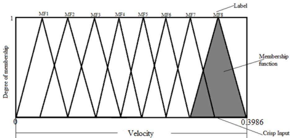
Fig. 8 Membership function for fuzzification of velocity
