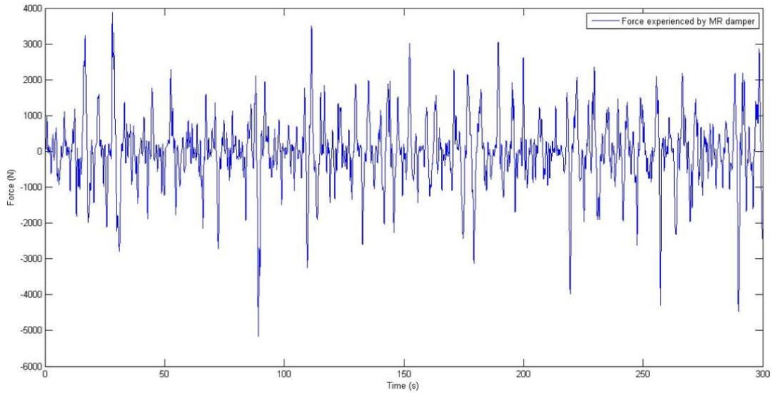
Fig. 14 Force acting on the MR damper at the 1<sup>st</sup> level
