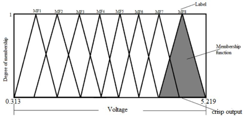
Fig. 9 Membership function for de-fuzzification of voltage
