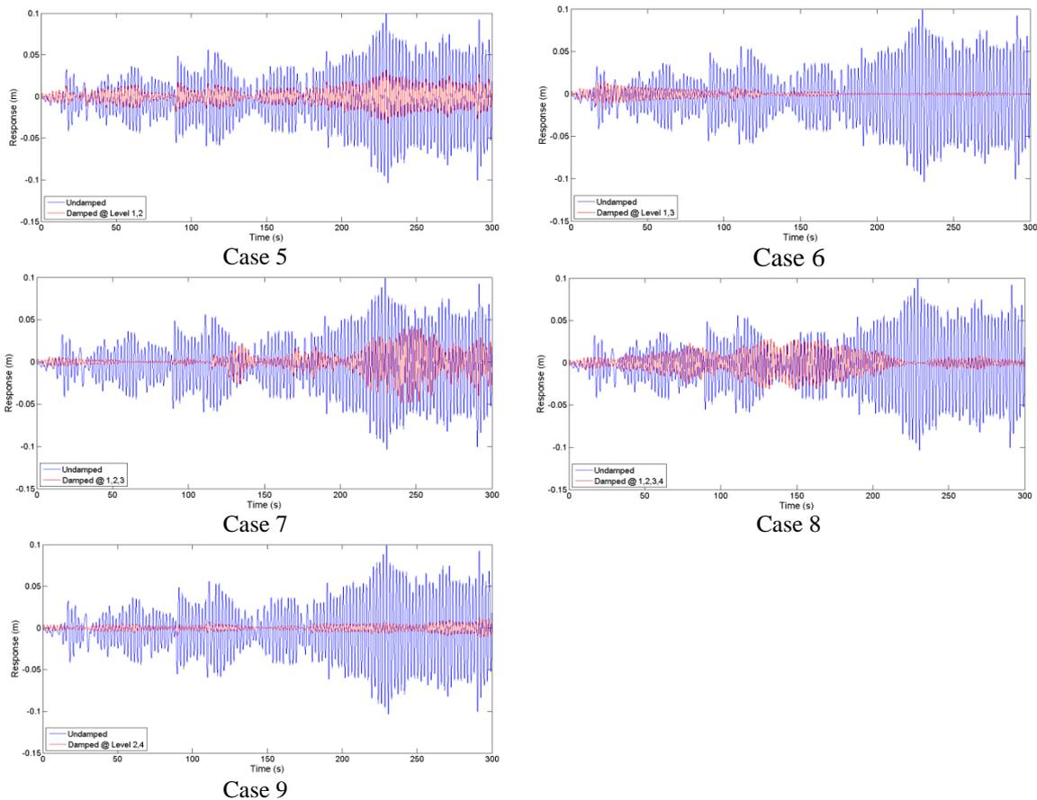
Fig. 16 MR damper placed at combination levels (cases 5,6,7,8 & 9)
