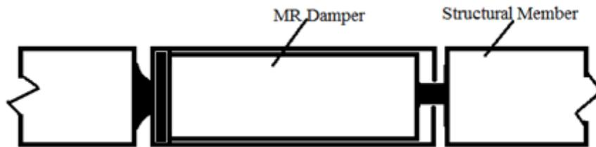
Fig. 10 MR Damper arrangement in structural member
