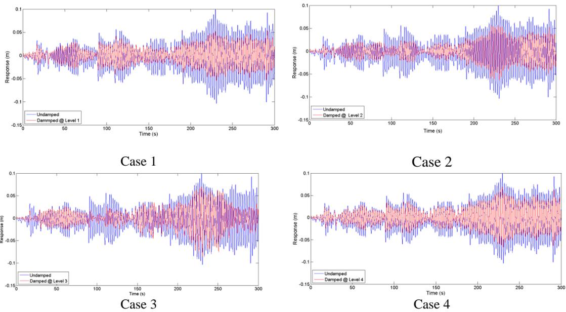
Fig. 15 MR damper placed at independent levels (cases – 1,2,3 &4)
