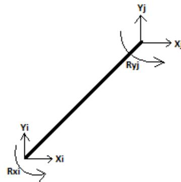
Fig. 4 Beam element in global coordinates
