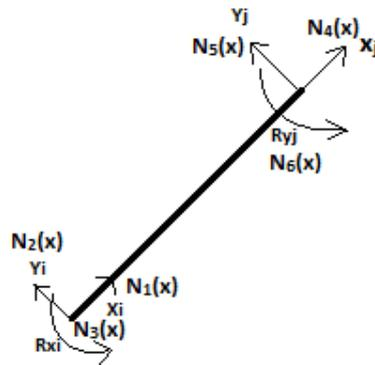
Fig. 3 Beam element in local coordinates
