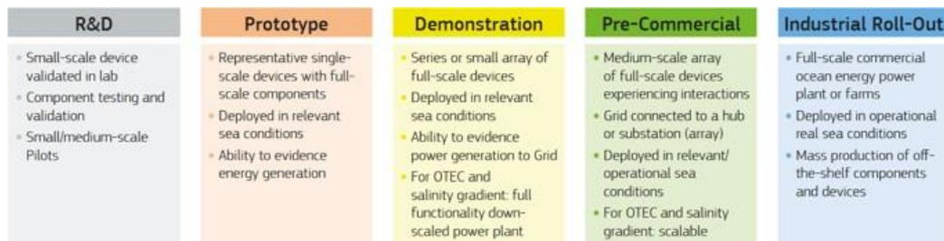
Fig. 28 Phases of Technology Readiness Level, (courtesy of Ocean Energy Europe. Generated through consultation with Ocean Energy Europe and the Ocean Energy Forum)
