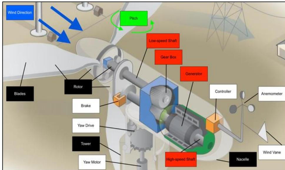
Fig. 4 Structure of a WTG, (U.S. Department of Energy, 2015)
