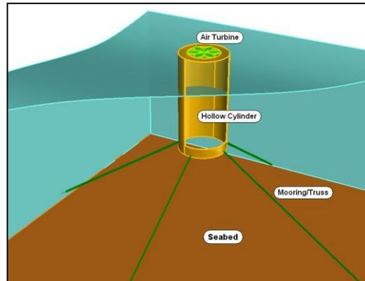
Fig. 17 Oscillating Water Column Principle (Wang and Falzarano 2017)
