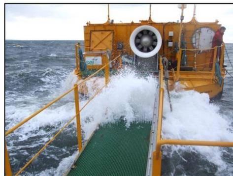
Fig. 18 Oscillating Water Column System, (Ocean Energy Limited, NREL 2005)
