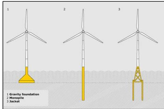
Fig. 11 Offshore WTGs Foundations, (courtesy of Züblin 2010)
