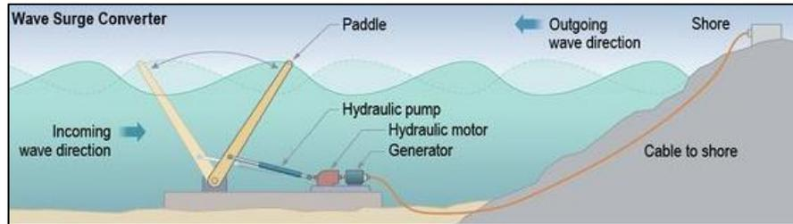
Fig. 19 Oscillating Wave Surge Converter, (OpenEI, NREL 2013)
