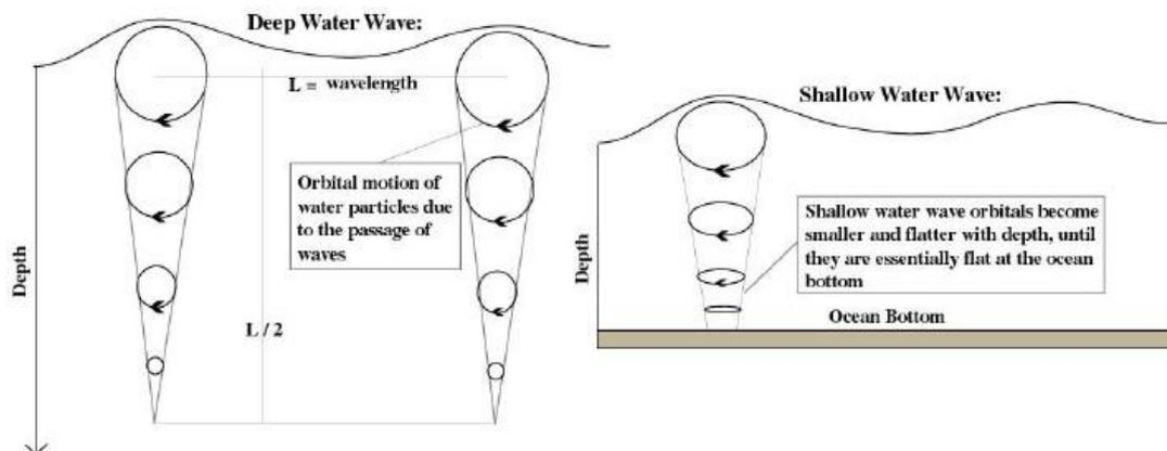
Fig. 16 Wave particle motion (State of New South Wales, 1990)
