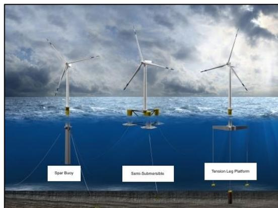
Fig. 12 WTGs Floating Solutions, (courtesy of DNV GL 2016)
