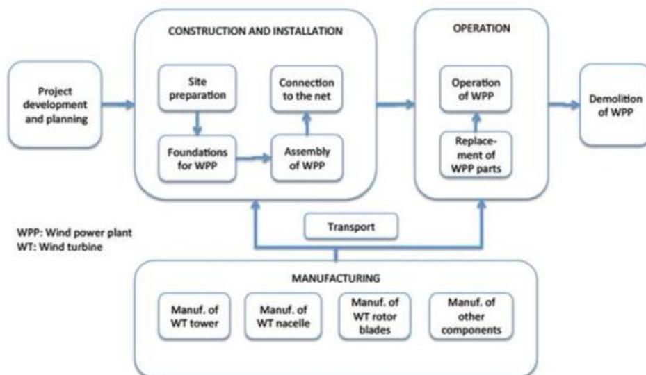
Fig. 29 Offshore Wind Supply Chain, (Breitschopf *et al.* 2011)
