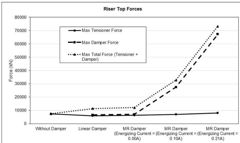
Fig. 13 Riser-top forces (Tensioner w/wo dampers)
