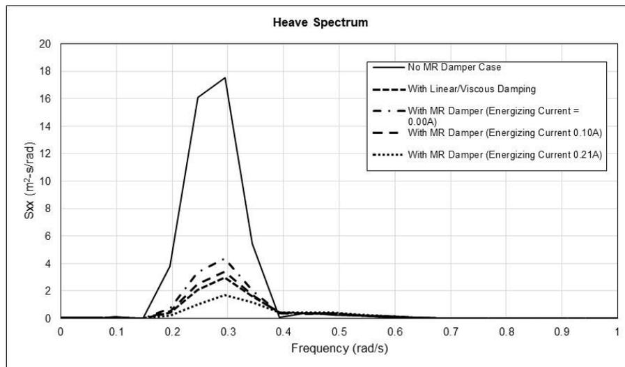
Fig. 11 Semisubmersible heave spectra (with and without damper)
