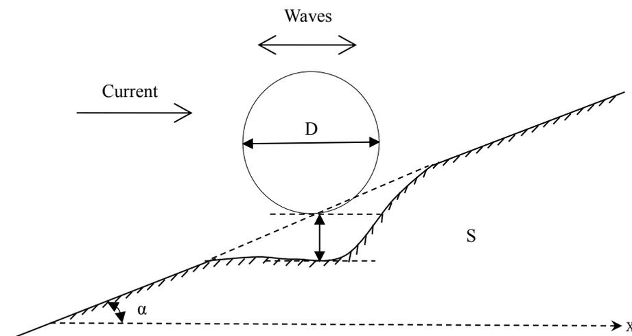
Fig. 2 Definition sketch of the scour depth ( $S$ ) below a pipeline with diameter ( $D$ ) on a mild slope ( $\alpha$ )
