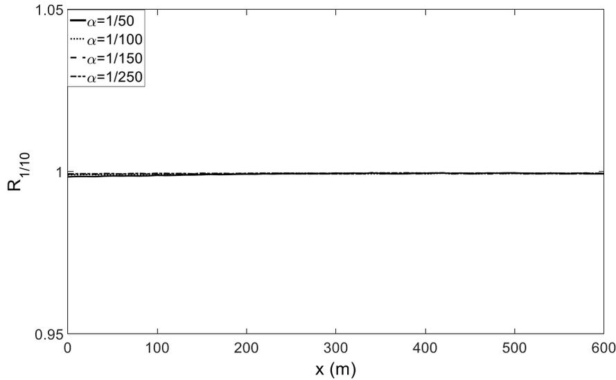
Fig. 12 Random waves alone: The stochastic to approximate method ratio  $R_{1/10}$  versus  $x$  for four slopes  $\alpha = (1/50, 1/100, 1/150, 1/250)$
