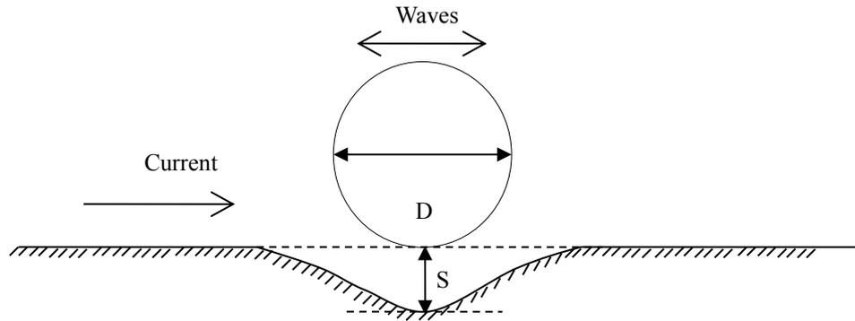
Fig. 1 Definition sketch of the scour depth ( $S$ ) below a pipeline with diameter ( $D$ )
