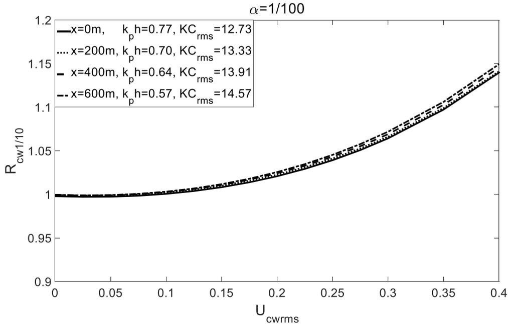
Fig. 13 Random waves plus current: The stochastic to approximate method ratio  $R_{cw1/10}$  versus  $U_{cwrms}$  at four locations for slope  $\alpha = 1/100$
