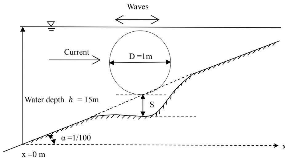
Fig. 3 Definition sketch of the seabed conditions with  $\alpha = 1/100$
