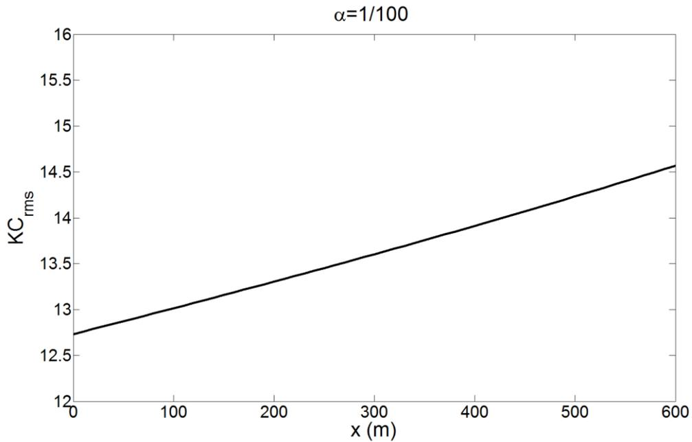
Fig. 5  $KC_{rms}$  versus  $x$  in finite water depth for slope  $\alpha=1/100$
