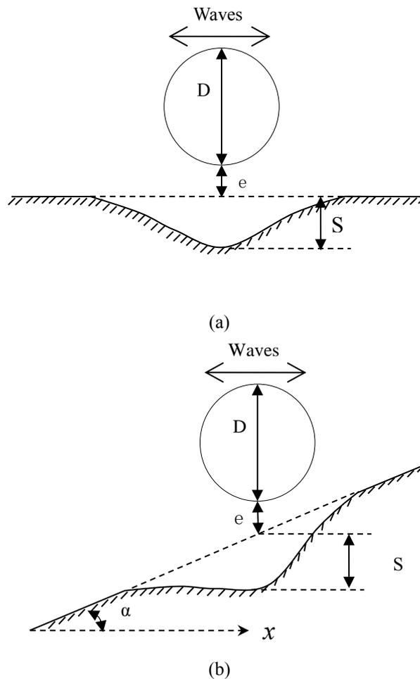
Fig. 14 Definition sketch of scour below pipelines with a pipe position  $e$  above the undisturbed bed: (a) on a horizontal bed; (b) on a mild slope
