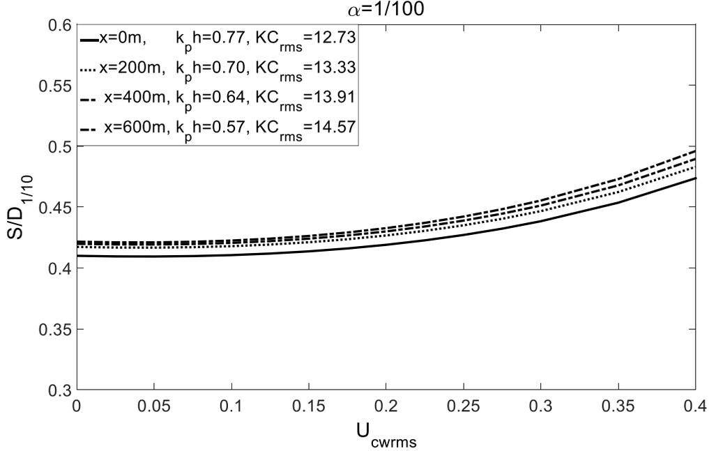
Fig. 11  $S/D_{1/10}$  versus  $U_{cwrms}$  at four locations for slope  $\alpha = 1/100$
