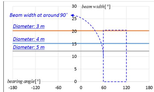
Fig. 15 Beam width of the circular array sonar
