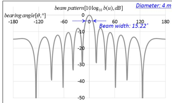
Fig. 6 Beam pattern of a circular array sonar (diameter: 4 m)
