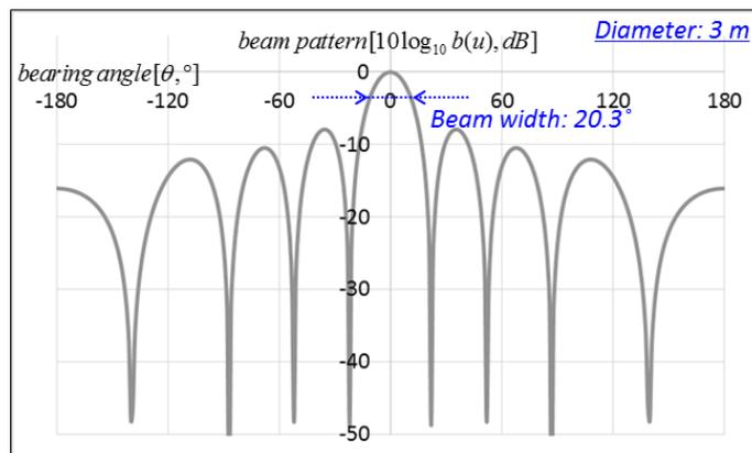
Fig. 5 Beam pattern of a circular array sonar (diameter: 3 m)
