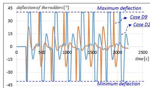
Fig. 27 Deflection of the upper rudder and the lower rudder in Cases D2 and D9
