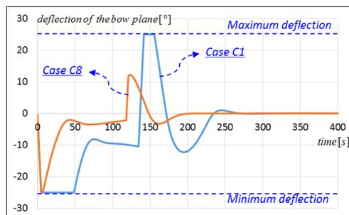
Fig. 21 Deflection of the bow plane in Cases C1 and C8
