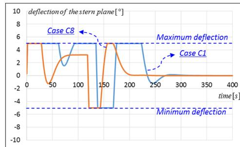
Fig. 22 Deflection of the stern plane in Cases C1 and C8
