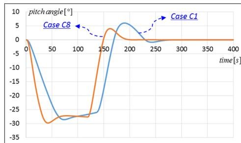
Fig. 20 Pitch angle variations in Cases C1 and C8
