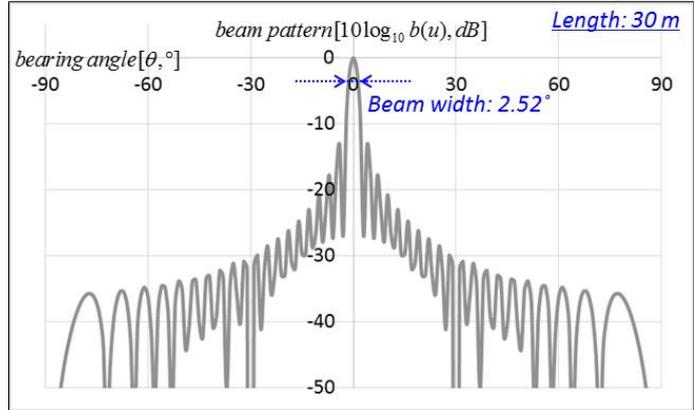
Fig. 9 Beam pattern of a linear array sonar (length: 30 m)
