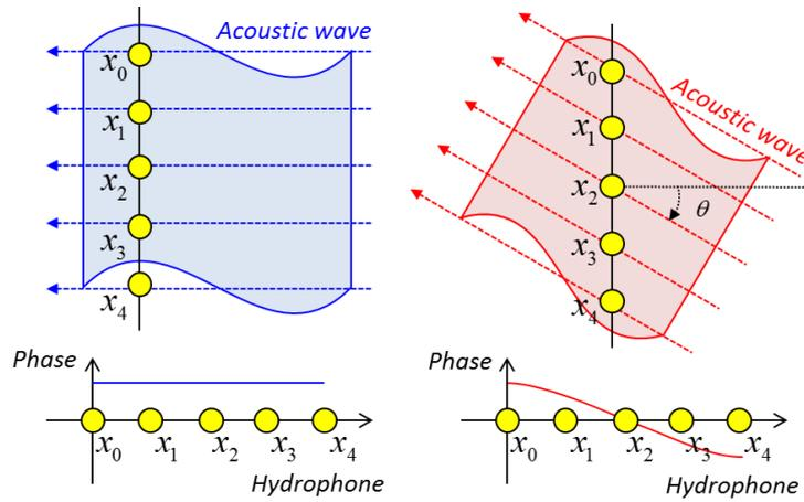
Fig. 2 Differences in the phases of the noise at each hydrophone
