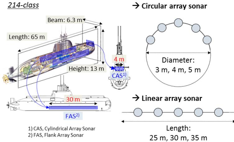
Fig. 4 Specifications of the passive sonars of a submarine
