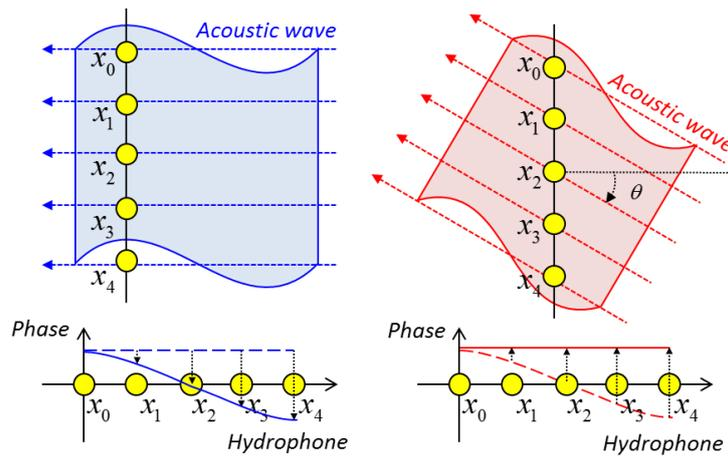
Fig. 3 Intentional differences in the phases of the noise at each hydrophone
