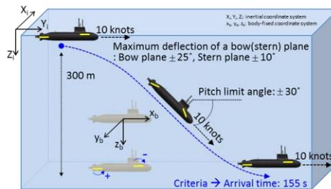
Fig. 18 First scenario for the maneuvering performance simulation
