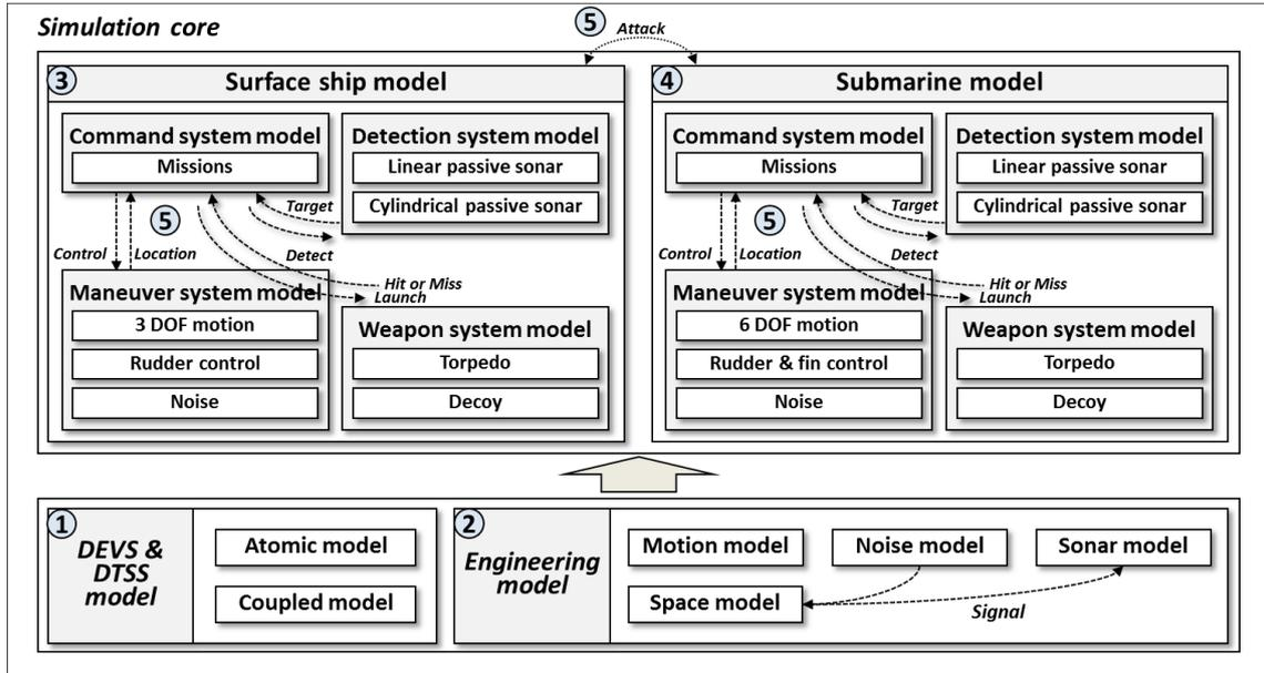
Fig. 1 Configuration of the simulation core and GUI
