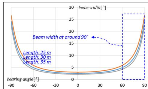
Fig. 16 Beam width of the circular array sonar
