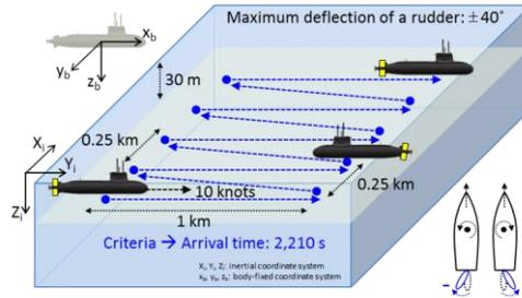
Fig. 24 Second scenario for the maneuvering performance simulation
