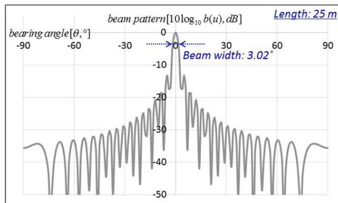
Fig. 8 Beam pattern of a linear array sonar (length: 25 m)
