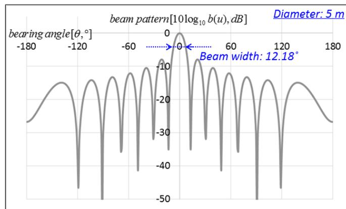
Fig. 7 Beam pattern of a circular array sonar (diameter: 5 m)
