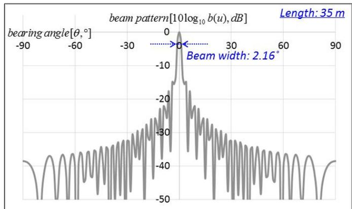
Fig. 10 Beam pattern of a linear array sonar (length: 35 m)
