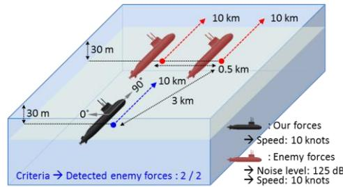
Fig. 14 Second scenario for the detection performance simulation
