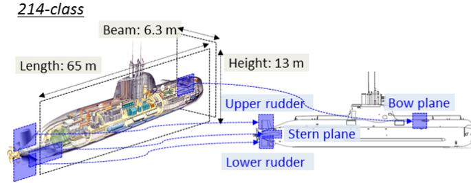
Fig. 17 Specifications of the hydroplanes of a submarine
