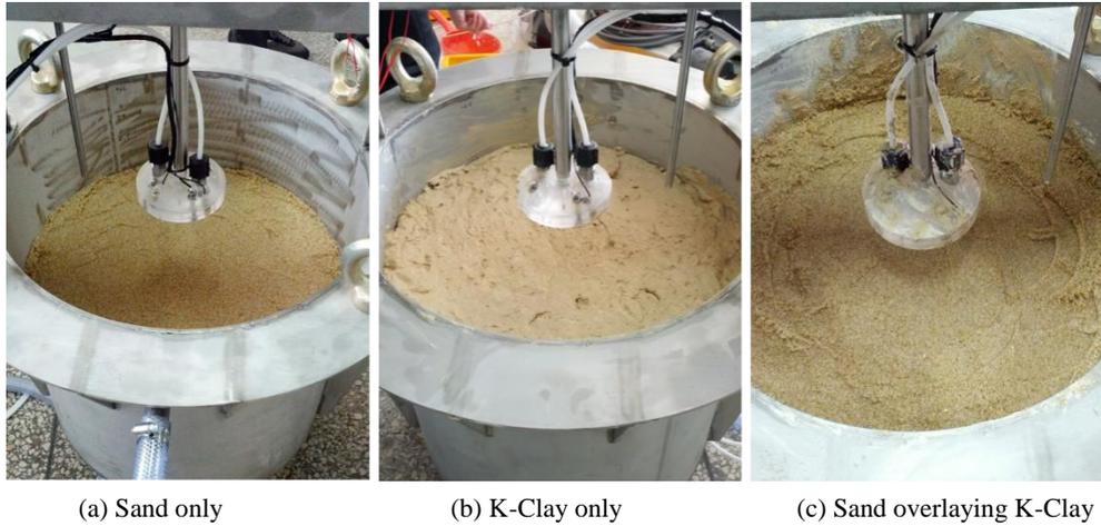
Fig. 2 Soil conditions for performance test
